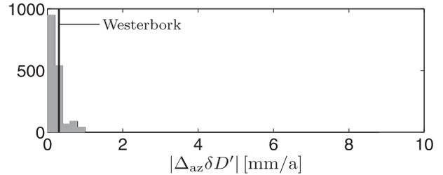
(b) Relative LOS displacement biases in azimuth that are induced due to approximation errors of the correction model (3).
