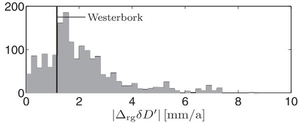
(a) Relative LOS displacement biases in range that are induced by the reference frame effect and can be removed with the correction in eq. (3).
