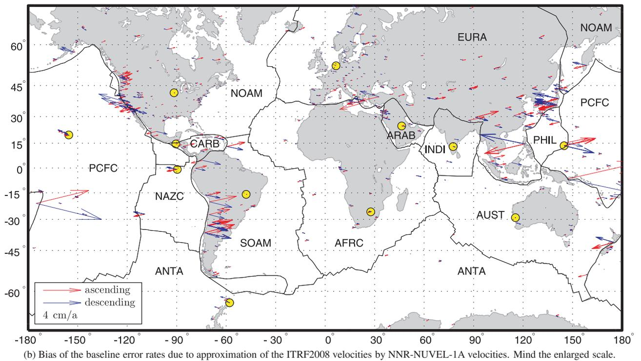
Figure 4: Prediction of the baseline error rate  $\delta B'_1 = v_\perp$  due to the reference frame effect for ENVISAT interferograms, evaluated at 840 ITRF2008 stations. The arrows are aligned to the horizontal projection of the respective radar line of sight. Numerical values for the twelve encircled stations can be found in tab. 1.
