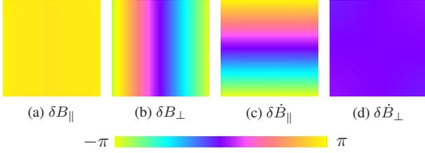
Figure 2: Interferometric error signals induced by errors in particular baseline components, computed for a full ENVISAT scene of  $100 \times 100$  km [7]. (a)  $\delta B_{\parallel} = 26$  cm. (b)  $\delta B_{\perp} = 26$  cm, equivalent to one fringe in range. (c)  $\delta \dot{B}_{\parallel} = 1.7$  mm/s, equivalent to one fringe in azimuth. (d)  $\delta \dot{B}_{\perp} = 1.7$  mm/s.
