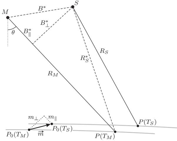
(a) Acquisition geometry in the ITRF datum.
