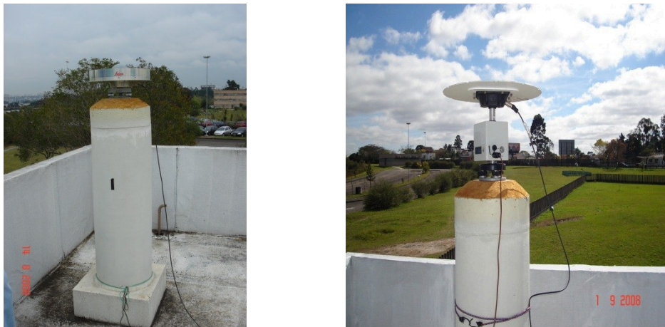
Figure 5: Relative field calibration at the BCAL/UFPR, left: reference antenna, right: DRB device and calibration antenna (KRUEGER ET AL., 2009).
