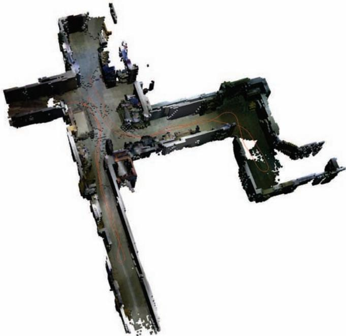
**Figure 5.1:** 3D voxel Map from SLAM with odometry and Kinect.
