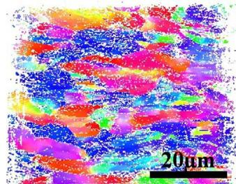
Figure 3.1: (a) EBSD results of a cross section prepared by FIB into the cold rolled DC04 steel.
