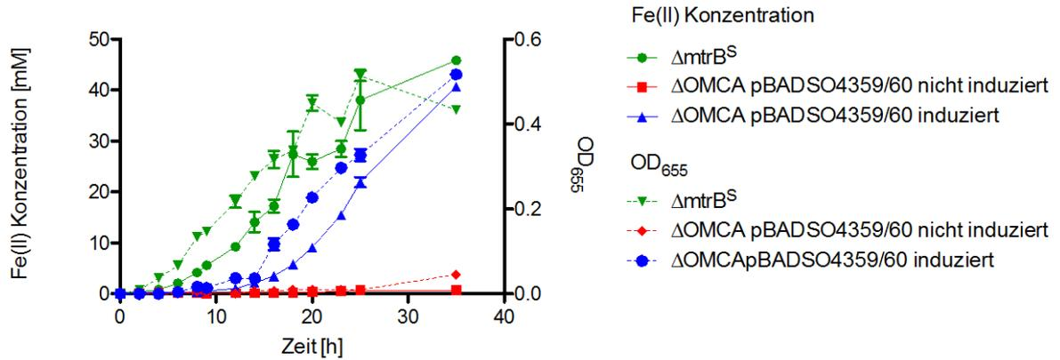
**Fig. 22)** Correlation between ferric citrate reduction (left y-axis, solid lines) and increase of the optical density (right y-axis, dashed lines) of similar grown  $\Delta mtrB^S$ , and induced or uninduced  $\Delta$ OMCA pBAD SO4360/59<sub>STREP</sub> strains on anaerobic 4 M minimal medium supplemented with 50 mM lactate and 50 mM ferric citrate. The assay was done over 35 hours.
