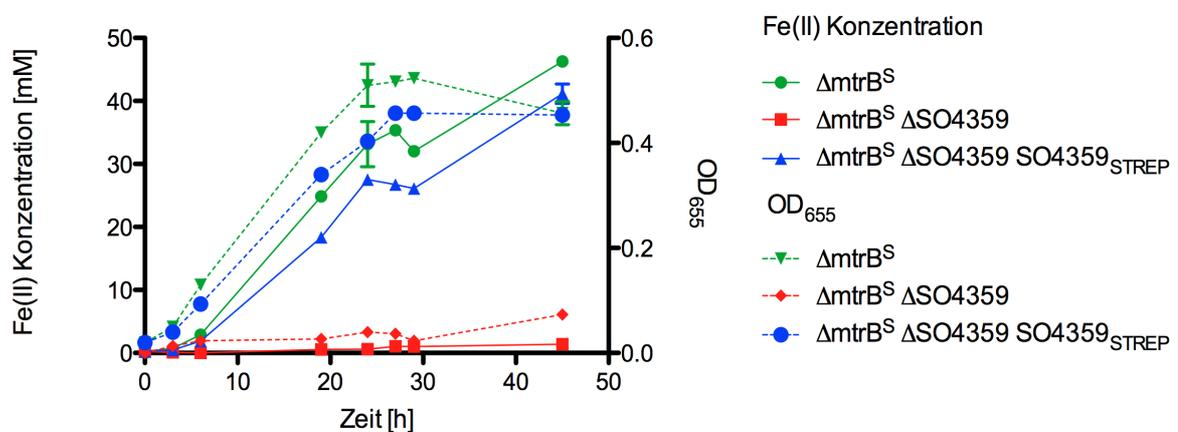
**Fig. 14)** Correlation between ferric citrate reduction (left y-axis, solid lines) and increase of the optical density (right y-axis, dashed lines) of similar grown  $\Delta mtrB^S$ ,  $\Delta mtrB^S$   $\Delta SO4359$  and  $\Delta mtrB^S$   $\Delta SO4359$  pBAD  $SO4359_{STREP}$  strains on anaerobic 4 M minimal medium supplemented with 50 mM lactate and 50 mM ferric citrate. The assay was done over 45 hours.
