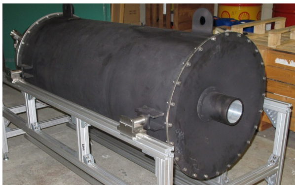
The stainless steel microwave load prepared for the second measurement in 2011.
