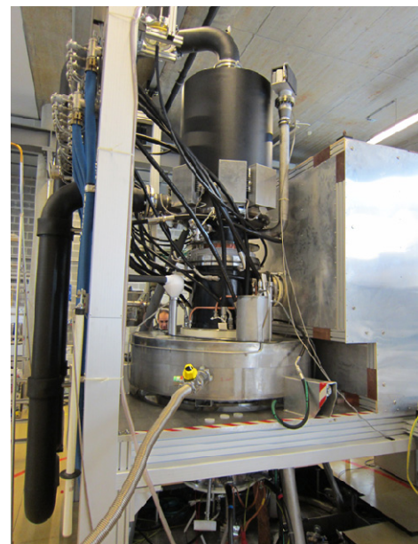
Coaxial 2.2 MW 170 GHz short pulse pre-prototype gyrotron at KIT (left); the refurbished industrial long pulse prototype at delivery end September 2011 (mid); and the same prototype, installed at the CRPP test stand inside the ASG magnet (right).
