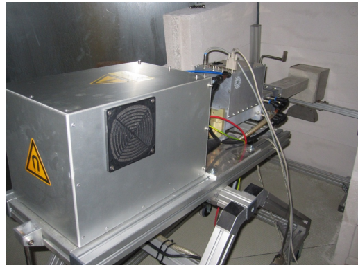
First prototype setup for microwave ablation of concrete.
