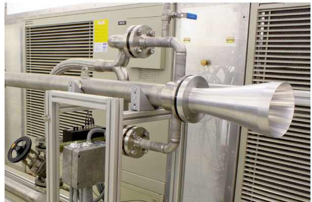
Input section of the long load, showing matching horn, and the absorbing waveguide with cooling connection.
