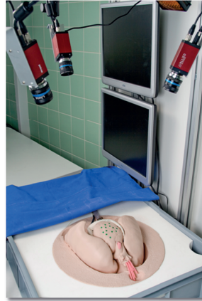
(b) The artificial beating heart is observed by a camera system.
