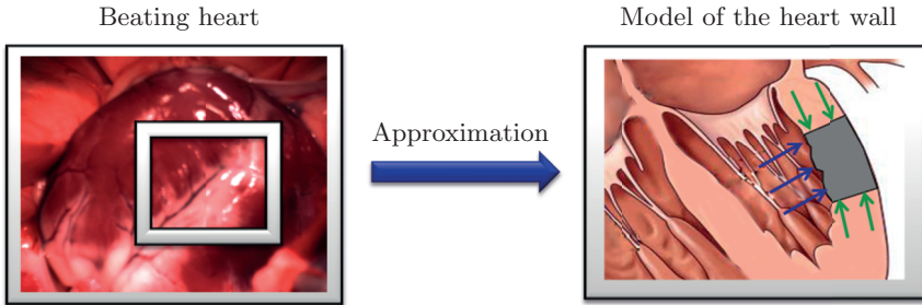
Figure 3.2: Approximation of the heart wall of the left ventricle by a heart model. The model considers the heart wall inside the operation area. This area is subjected to the external forces, such as pressure forces inside of the cardiac chamber (blue) and muscle forces (green).
