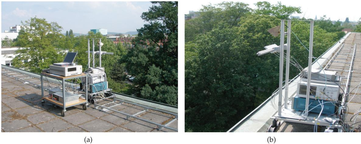
Figure 7.3.: Photos of the demonstrator for the ground-based SAR experiment: (a) the set-up of the demonstrator on the test site and (b) the side view to indicate the sensor position close to the edge of the building and the look angle.
