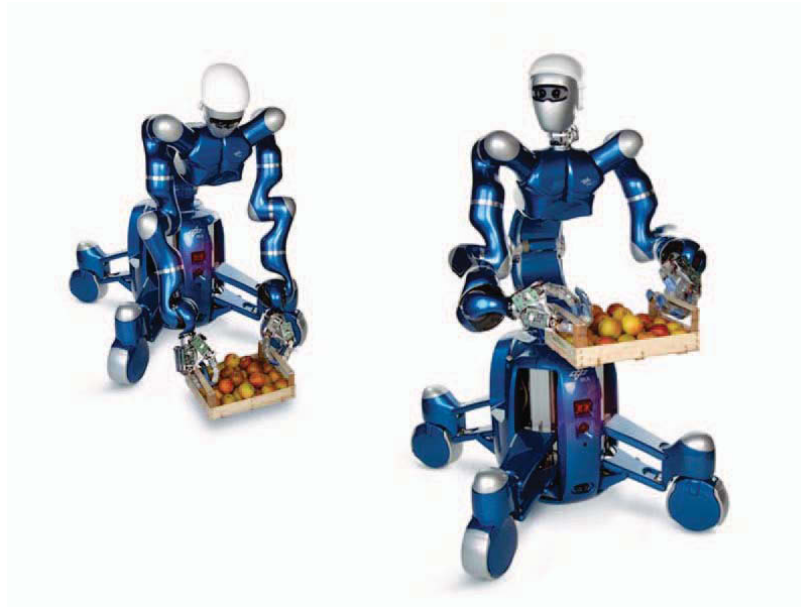
Figure 1.4: The DLR Justin, a humanoid robotic system for service robotics in unstructured environment, e.g. Ott et al. [114]
