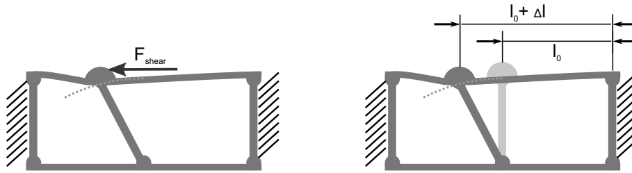
Figure 3.46: Deviation of the strain sensitive structures as a result of the geometry of the surface structure.
