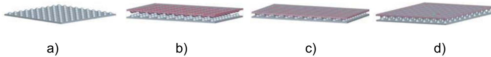
Figure 3.60: The manufacturing process of the polymer spacers is adapted from the packaging of integrated circuits where ball grid array chips are mounted upside down on the surface of printed circuit boards. The basic polymer substrate is provided with polymer dots with defined material volume, e.g. by screen printing (a). Subsequently two basic substrates equipped with polymer dots are opposed (b) and connected (c). Finally the polymer of the spacers is fixated (d).
