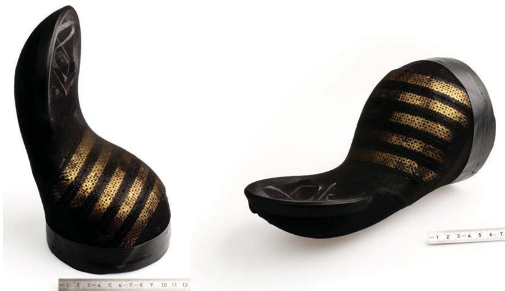
Figure 3.76: Front and side view of a prototype of a normal force acquisition tactile surface sensor with 5 \times 8 taxels. The spatial resolution of the prototype is 20\text{mm} . While the spatial resolution is comparatively low, the design of the tactile surface sensor enables the reduction of the insensitive surface area. The sensitivity of the tactile surface sensor is independent of the location of a contact within the surface area of an individual taxel.
