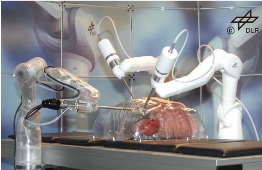
Figure 1.5: The DLR Mirosurge setup for robotic minimally invasive surgery, e.g. Hagn et al. [49]
