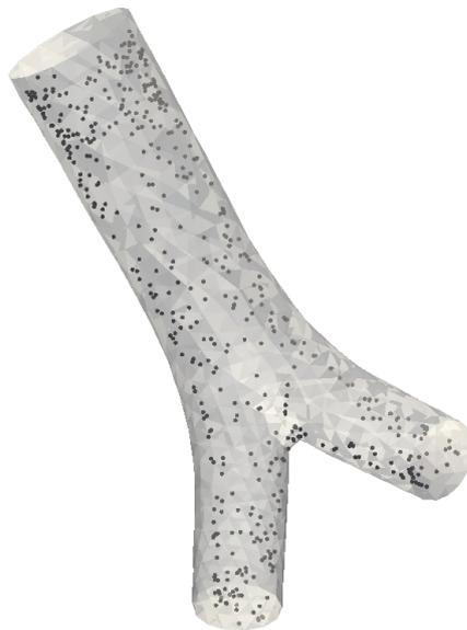
Figure 1.3: Particles flowing through one schematic bifurcation. We show that we can plug together these building blocks, parametrized bifurcations, with respect to some patient-specific geometrical parameters and obtain significantly similar results to the full patient-specific simulation.
