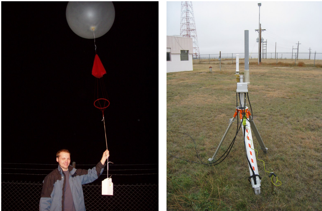
Figure 5.4: Left: A weather balloon with parachute (red, middle) and radiosonde (white, bottom). Right: Ground equipment used in Colorado. The GPS antenna is the smaller, white antenna on the left, the receiving antenna in gray on the right side of the tripod. The white box mounted below the antennas is a signal amplifier.
