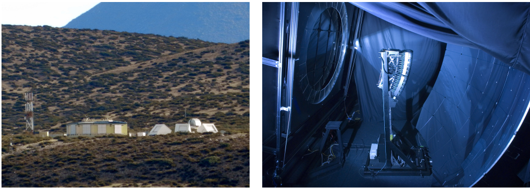
Figure 3.3: The Fluorescence Detector (FD). On the left, the FD site at Coihueco with the more recent HEAT telescopes in the foreground and a LIDAR station in the background. The inside of a telescope is shown on the right. The light enters through the aperture at the left and is reflected off the mirror onto the PMT camera in the middle.
