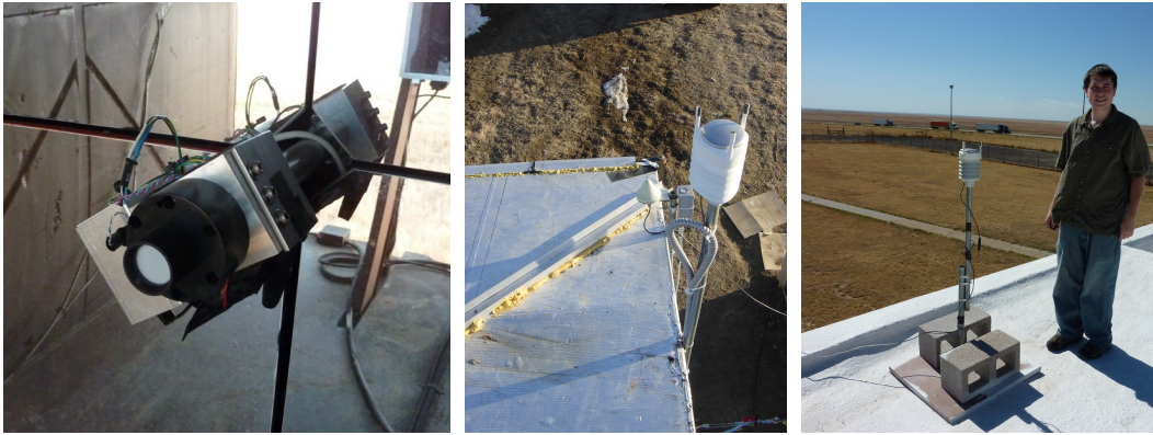
Figure 8.11: On the left, the calibration LED that is used between runs for a relative calibration of the AMT pixels. In the middle, the weather station at the AMT can be seen, below the station is a cloud monitor and the GPS antenna. On the right, the DRLF weather station is shown.
