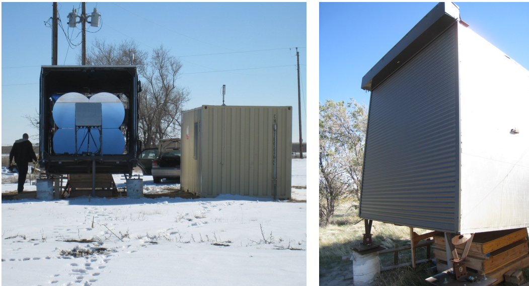
Figure 8.5: On the left, a picture of the AMT and the support container. The telescope includes the mirror and the camera, weather sensors and a calibration system. The container is equipped with internet access and houses the data acquisition electronics, the single-board computers to steer the operations and a personal computer as gateway and for manual access. The power and data connections between both are underground. The old door design with two outward swinging doors can be seen. The new rolling door design is shown on the right.
