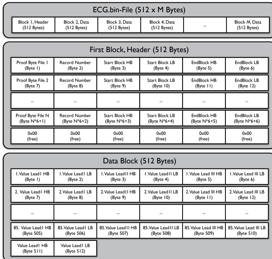
Fig. 4.8. Schematic description of the data file "ECG.bin"
