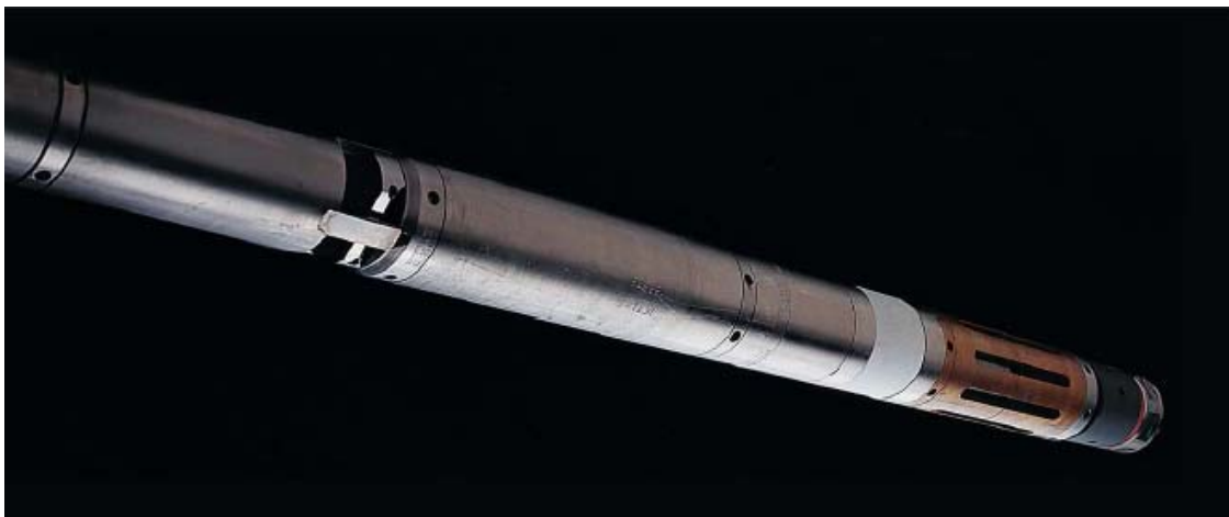
Figure 18 : CBIL tool; adapted from [BakerHughes, 2004]
