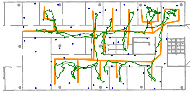
Figure 9.8: ITI: Tracking result using the force-directed approach without step recognition. The orange path shows the reference trajectory, the green path shows the computed trajectory.
