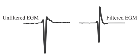
Fig. 9.8: Effect of applying a band-pass filter (30–150 Hz) on electrograms (adapted from [135]).
