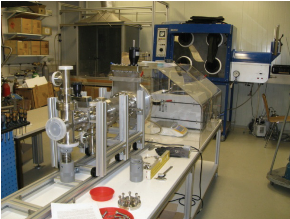
Fig. 2: Modified facility to measure hydrogen release due to Be-substitute/steam reaction at high temperatures and low pressures.
