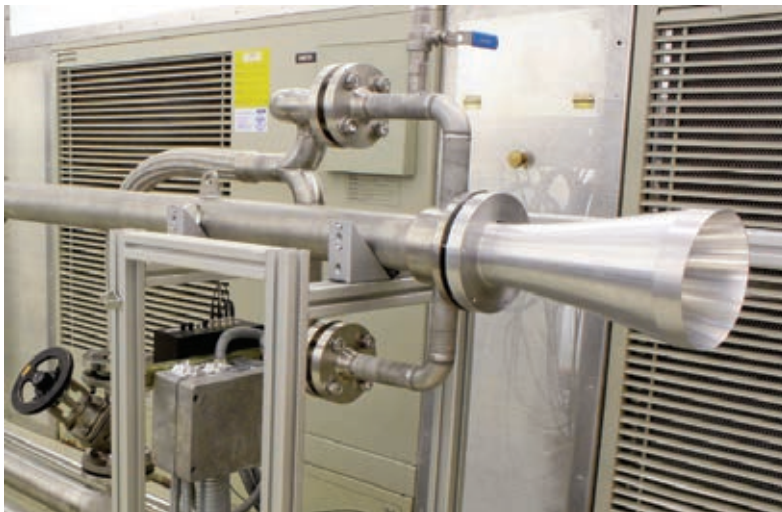
Fig. 4: Input section of the long load, showing matching horn, and the absorbing waveguide with cooling connection.
