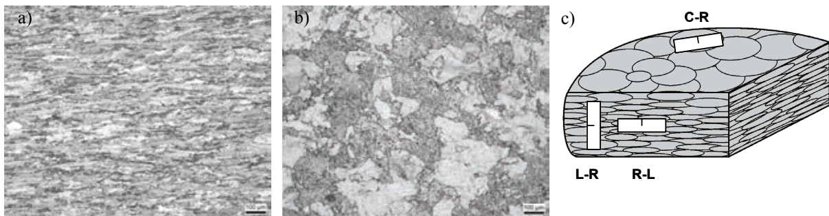
Fig. 1: Microstructure of polycrystalline round blank tungsten a) plane transverse to base; b) plane parallel to base; c) specimen orientations for the study of the influence of anisotropy on the fracture toughness.
