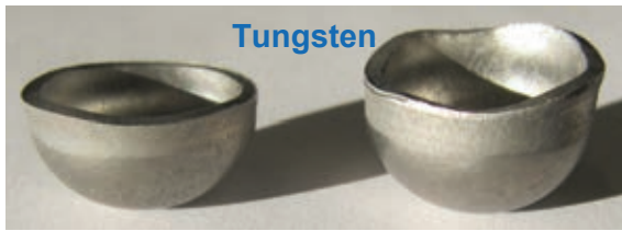
Successful deep draw attempts from 1 mm thick tungsten sheet for mass production of divertor thimble ( \varnothing 15 \times 1 ).
