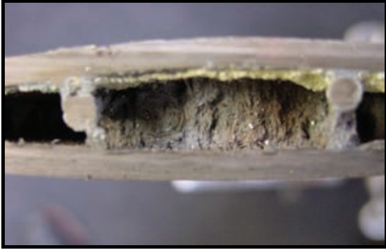
Plugging of the electro-magnetic pump by precipitates.
