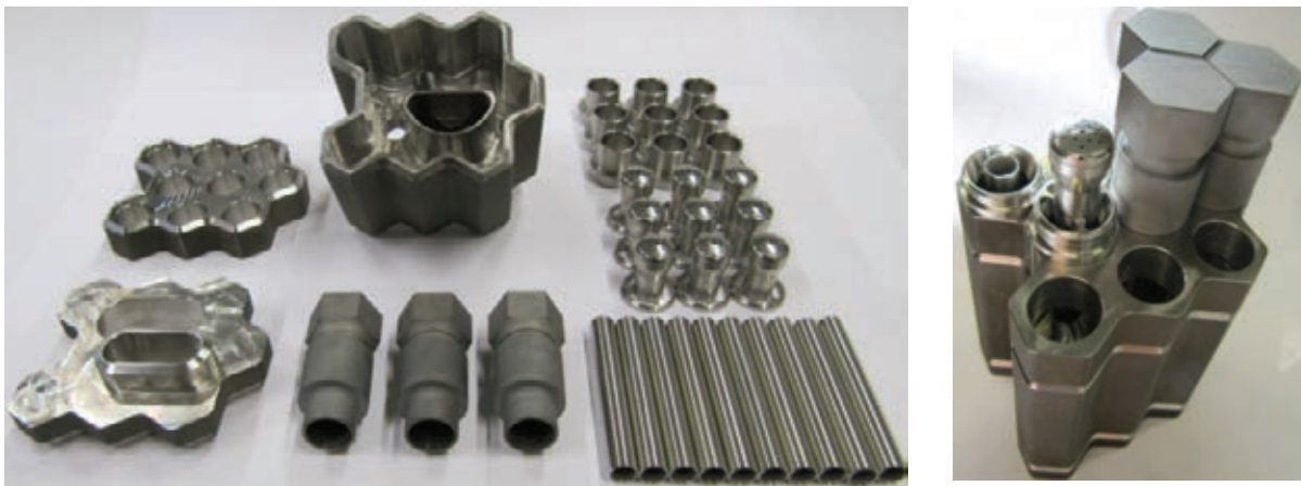
Fig. 1: 9-finger module manufacturing. Left: individual parts, right: assembly view.
