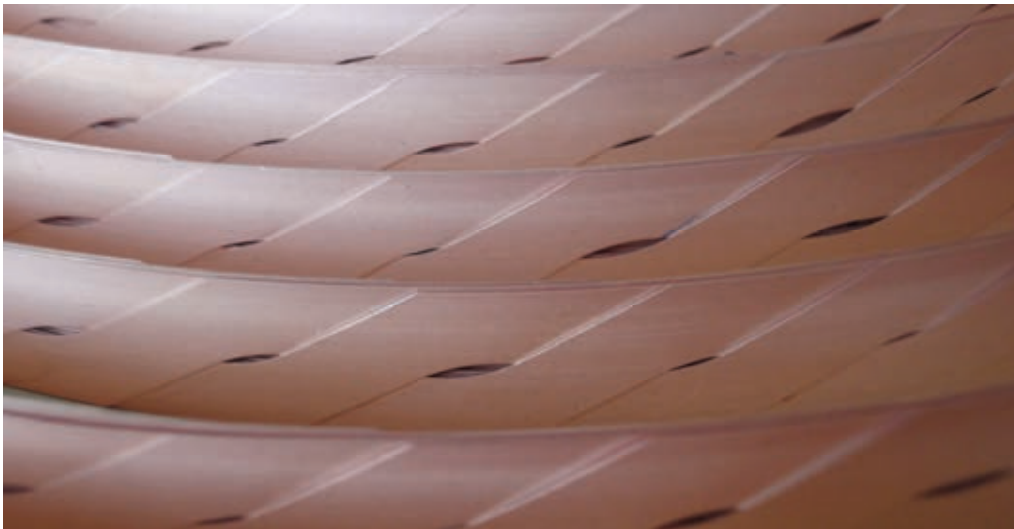
Fig. 4: Long length of a Roebel cable with 4.5 m, 10 strands and 12 mm width.
