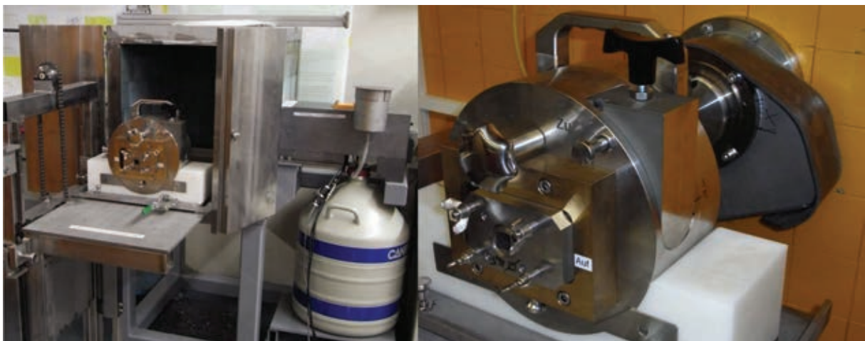
Fig. 3: Gamma spectrometer with shielding device for specimen and detector (left), transport unit for transfer from Hot Cell (right).
