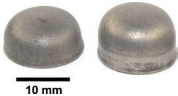
Fig. 3: Left: a blank with a diameter of 23 mm leads to a deep drawn thimble with a height of 8 mm. Right: a diameter of 26 mm leads to a height of 10 mm. Deep drawing was performed in a high vacuum at 600°C.
