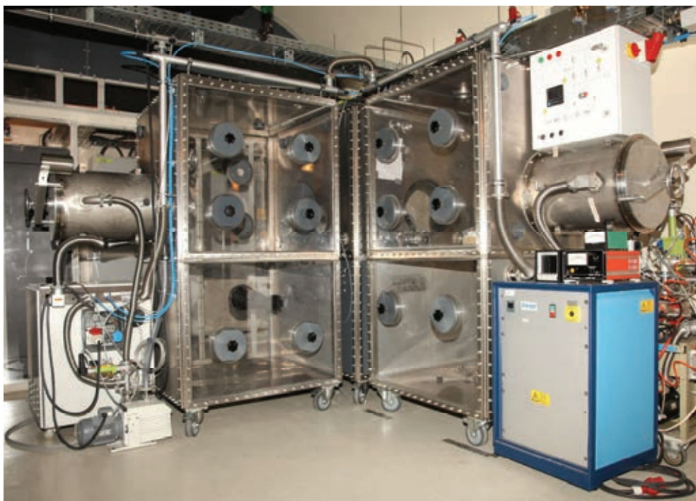
Fig. 1: New glove-box system consisting of three sections (the third section is in the background).
