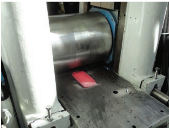
Fig. 2: Rolling of the 1 kg slabs in a 1,800 kN 12 inch Duo Mill (left) and partitioning of rolled plate for specimen fabrication (right).
