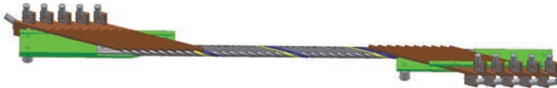
Fig. 6: CAD drawing of the sub-size CCRC demonstrator cable.
