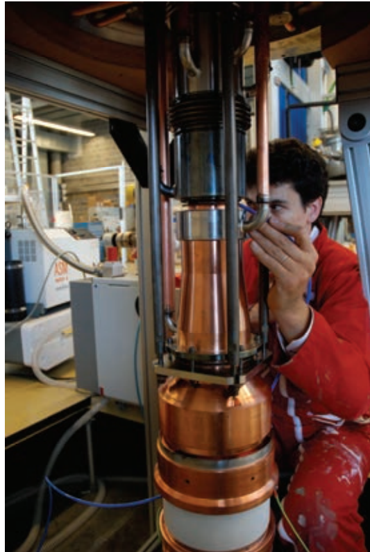
Fig. 2: C. Lievin (TED) fixing the vacuum leak.
