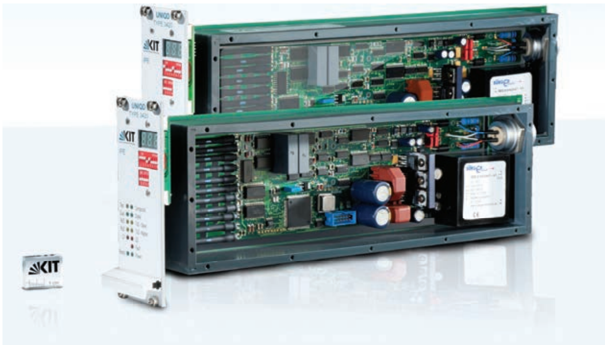
Fig. 1: Revised KIT-Quench detector UNIQD TYPE 3420.
