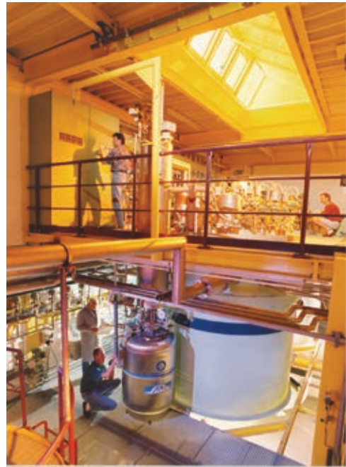
Fig. 1: 2 kW-refrigerator with valve box and calorimeter.
