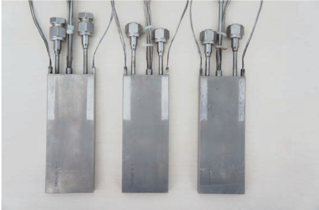
Fig. 2: Three fabricated capsules filled with specimens for irradiation in the BR2 MTR reactor.
