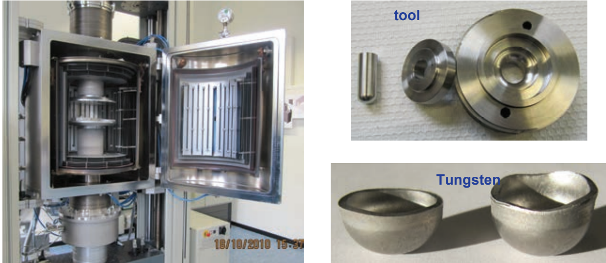
Fig. 1: Successful deep draw attempts from 1 mm thick tungsten sheet for mass production of divertor thimble ( \text{Ø}15 \times 1 ).
