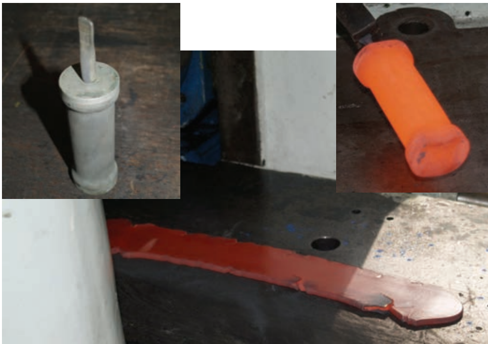
Fig. 3: Capsules after HIPping, and during hot-rolling.
