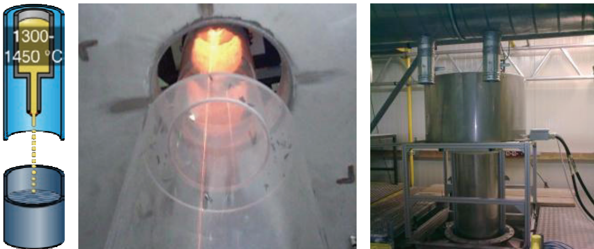
Fig. 1: Experimental setup – test facility (drawing), single nozzle beam and the new oven.
