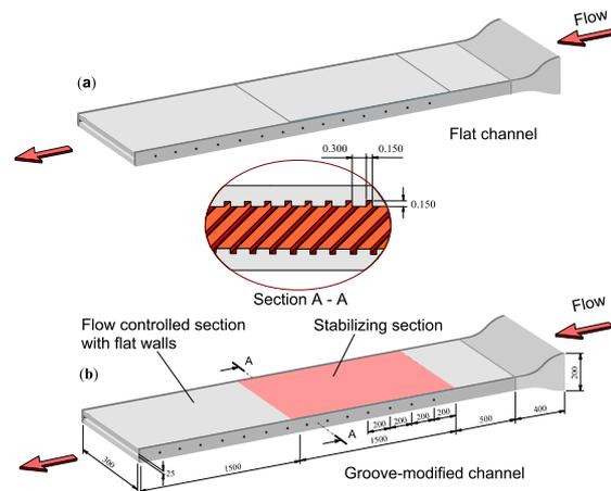
Figure 3: Two-dimensional channel flow with flat and groove-modified test section arrangements. (a) Reference test section configuration. (b) Configuration of the test section for laminar flow control.
