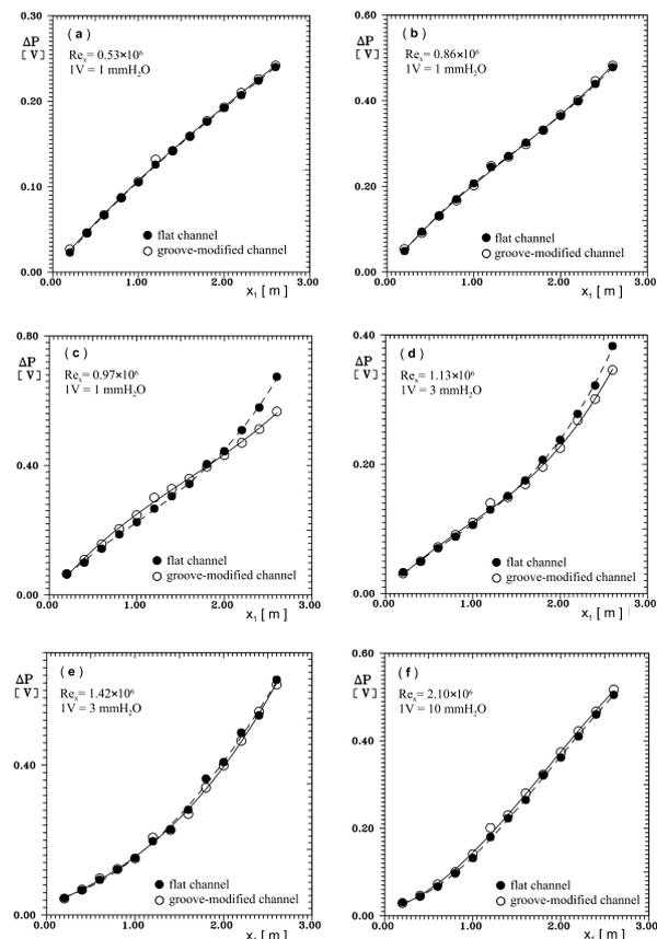
Figure 5: Comparisons of pressure drop distributions measured over flat and groove-modified test sections at different Reynolds numbers. The Reynolds numbers are based on the bulk velocity and the test section length.
