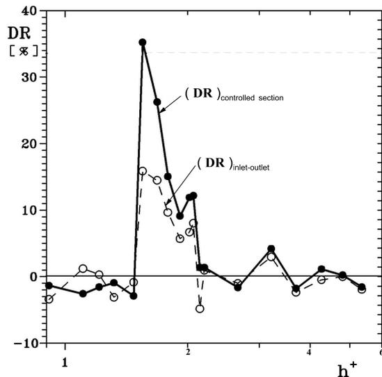
Figure 7: Drag reduction versus non-dimensional groove height:  $(DR)_{\text{controlled section}}$ , drag reduction measured over the flat part of the groove-modified test section;  $(DR)_{\text{inlet-outlet}}$ , net drag reduction measured over the entire length of the groove-modified test section.
