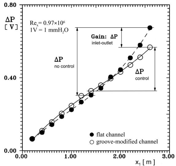
Figure 6: Comparison of pressure drop distributions in flat and groove-modified test sections for maximum drag reduction effect.
