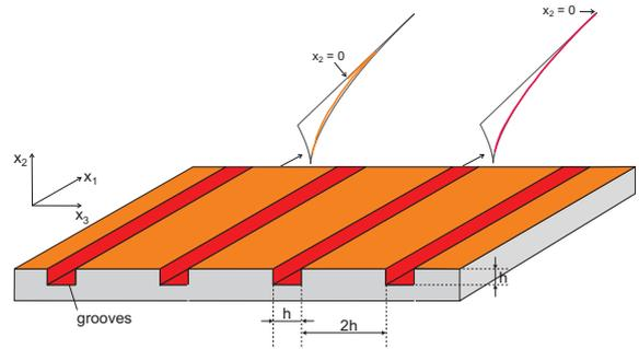
Figure 2: Surface topology capable of producing a smart interface between the flowing fluid and the solid boundary which promotes a large viscous drag reduction under particular circumstances: grooves are inserted in the wall and are aligned in the flow direction with the aim of forcing turbulence in the grooves towards the one-component limit. Sketched are the expected trajectories across anisotropy-invariant maps for each portion of the surface.
