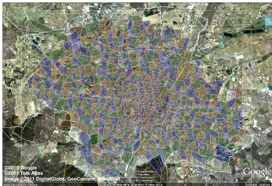
Figure A.4: Google Earth™ screenshot of a cellular network approximation via a Voronoi diagram (represented as KML file) as provided on the cellular analysis paper [3] website. Cell sizes in different city regions become obvious.
