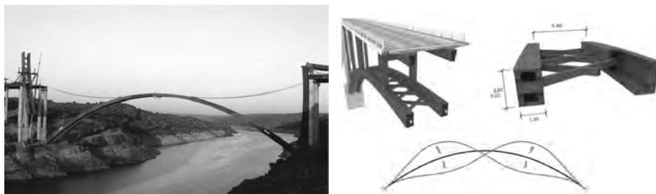
Fig. 1 The Alconétar Bridge: overview during erection (left), diagram of the whole unit formed by arch, metal piers and deck (top, right) and antimitriral vibration mode (bottom, right) [1]
