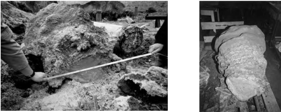
Fig. 2 The jet-grouting column excavated in the building site (left) and in the laboratory after cleaning (right) (J. Bzówka [1])
