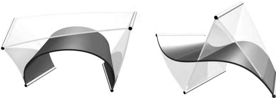
Fig. 4 Subdivision scheme for ruled surfaces (grey) with helicoids (transparent), control lines (orange) of third degree.
