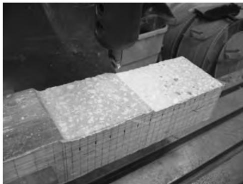
Fig. 1 Sectional milling of concrete prism.
