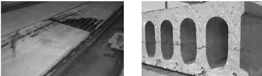
Fig. 3 Damaged slabs caused by the stopped tensed concrete sawing blade (left). Horizontal cracked webs of a slab caused by the tensed concrete sawing blade (right).
