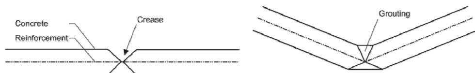
Fig.1 Sketch of the principle of folding: (left) before folding, (right) after folding and fixing
