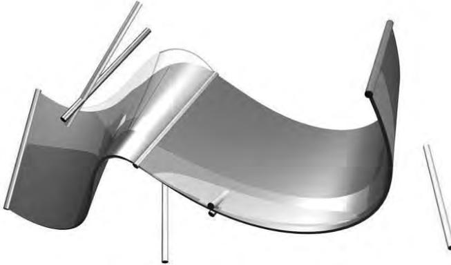
Fig. 7 Modification of the screw parameter results in new control lines (blue); ruled surface (grey); initial ruled surface (transparent), cf. fig. 5 (grey).
