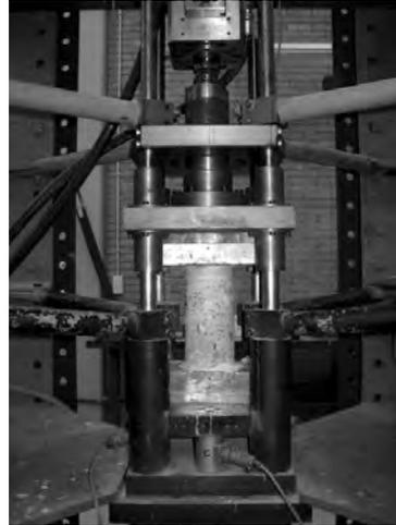
Fig. 1 Al-Kubaisy and Young sustained loading test principle and setup of axial tensile test
