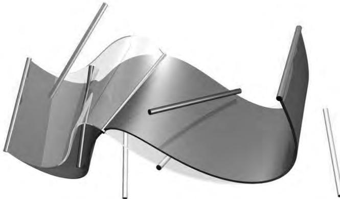
Fig. 6 Modification of the bias yields new control lines (blue); resulting ruled surface (grey); initial ruled surface (transparent), cf. fig. 5 (grey).
