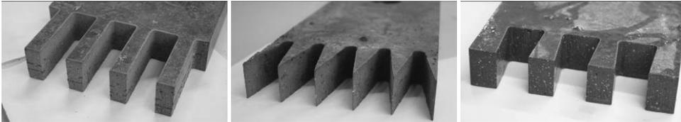
Fig. 1 The three different joint geometries, a) geometry A: rectangular teeth, b) geometry B: triangular teeth, c) geometry C: undercut geometry with pre-wetted surface
