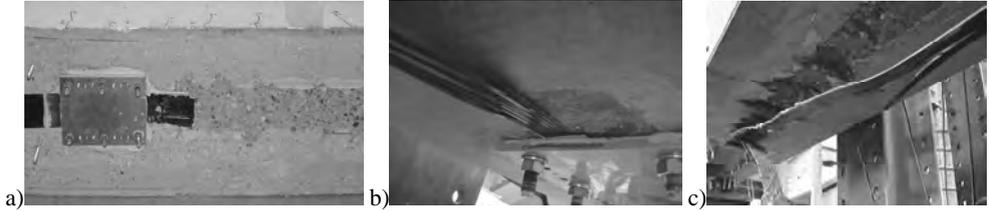
Fig. 3 View of bottom side after beam failure in the beams: a) P1, b) P4, c) P2.
