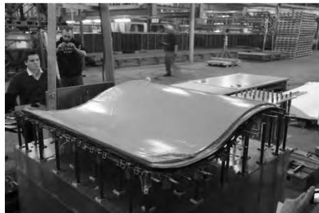
Fig. 15 shows a FRC panel on the flexible mould.
