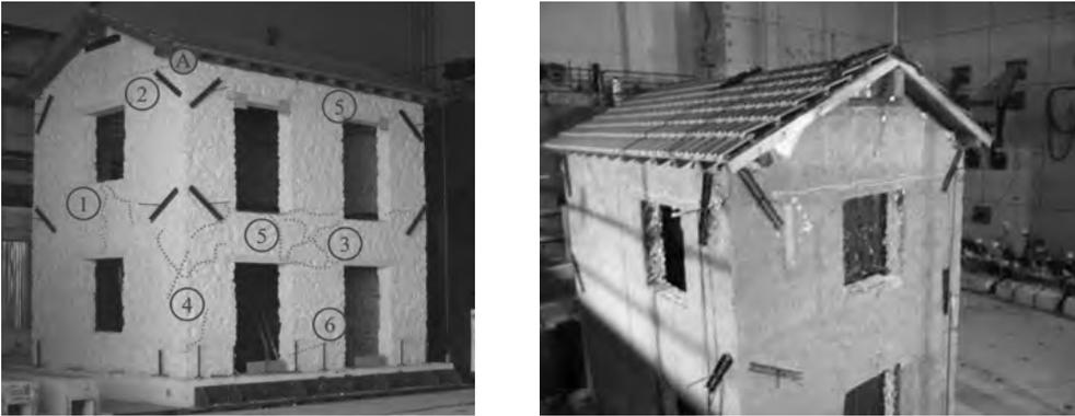
Fig 8 Cracked URM building (left),
