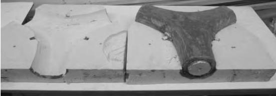
Fig. 5.3 Retracted prototype-node and elements of the mould made from expanded polystyrene
