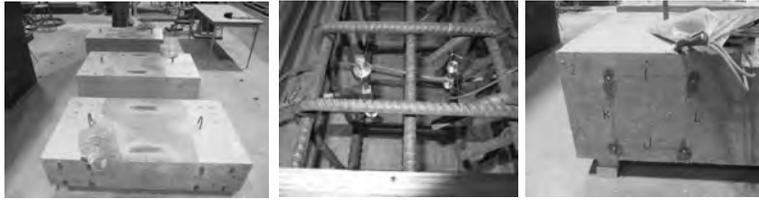
Fig. 1 Slab which is equipped by expansion measurement instruments. Left: concrete slabs fabricated in laboratory; middle: internal instrumentation for expansion measuring; right: concrete slabs equipped by pins for expansion measuring by Demec.
