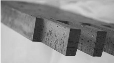
Fig. 2 Detail of the surface of the teeth cut with the water jet technique
