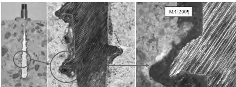
Fig. 1 Cross-sectional view of a mortared screw anchor after installation
