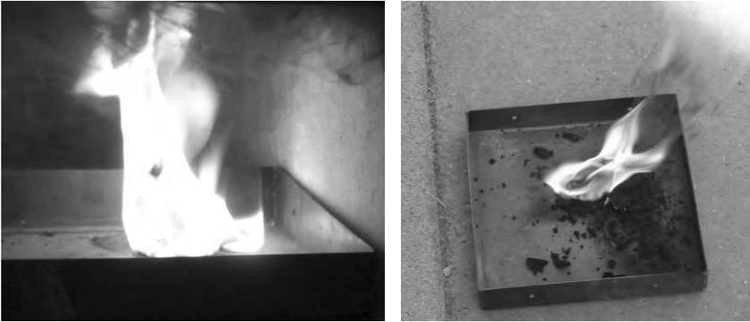
Fig. 3 Burning of UP polymer concrete specimens (left and right)
