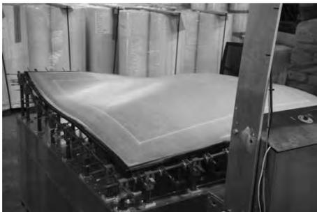
Fig. 14 shows a machine which can produce flexible surface
