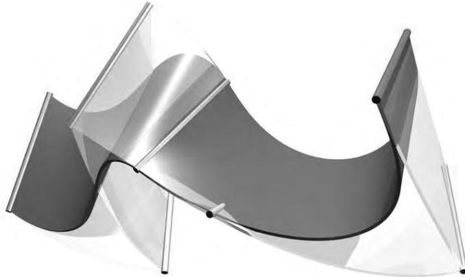
Fig. 5 Subdivision scheme for ruled surfaces (grey) with helicoids (transparent), control lines (orange) of third degree.
