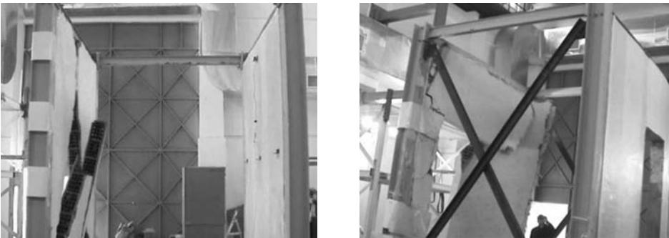
Fig. 6 URM wall without opening is collapsing URM wall with opening is collapsing (right)
