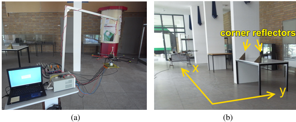
Figure 6.5: Setup of Airquad-borne SAR measurements: (a) setup of system; (b) geometry of measurements, where the system moved along the positive x axis (azimuth direction).
