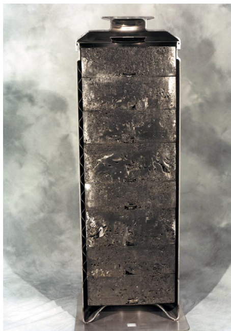
Fig. 14 Supercompacted hull and end pieces discs stored in a standard canister [135].
