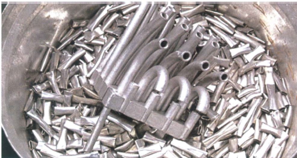
Fig. 13 Compaction of hulls and end-caps from spent nuclear fuel assemblies [135]
