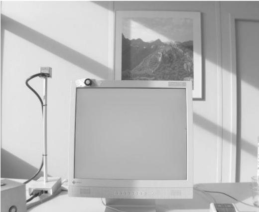
Figure 5–11: Monitor under daylight condition. As visible in this image the direct light from the outside is reflected on to the screen. Even such extreme cases are considered in the experiment to provide a dataset including all possible conditions for evaluation.
