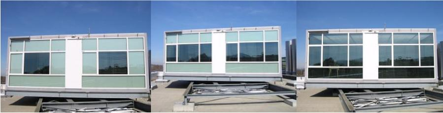
Figure 3–2: Images of the test rooms with the three window sizes (left - small size window, middle- medium size window, right – large size window) [83].
