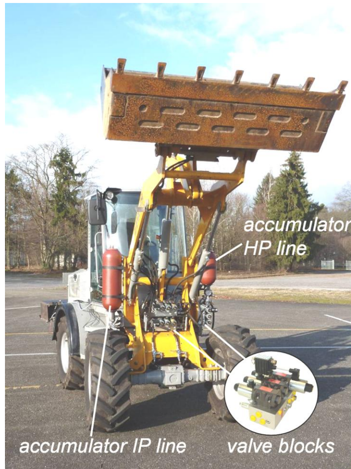
Figure 8: Test machine with mounted valve blocks and accumulators
