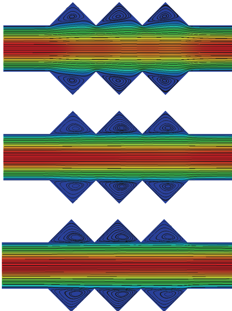
Figure 5: Steady flow in the zig-zag geometry with Re = 100 (upper), Re = 500 (middle), and Re = 1,000 (lower).
