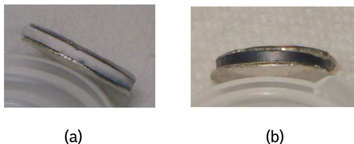
Figure 4.29. Pellets processed in air after contact with Li-metal for (a) 1 day and (b) 7 days
