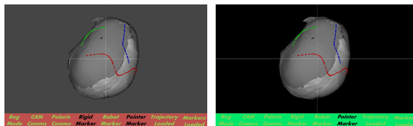
(a) GUI of System showing a problem. The rigid marker cannot be seen by the tracking system. (b) GUI of Functioning System, with Registration complete, robot and rigid body visible to optical tracking and all components loaded
