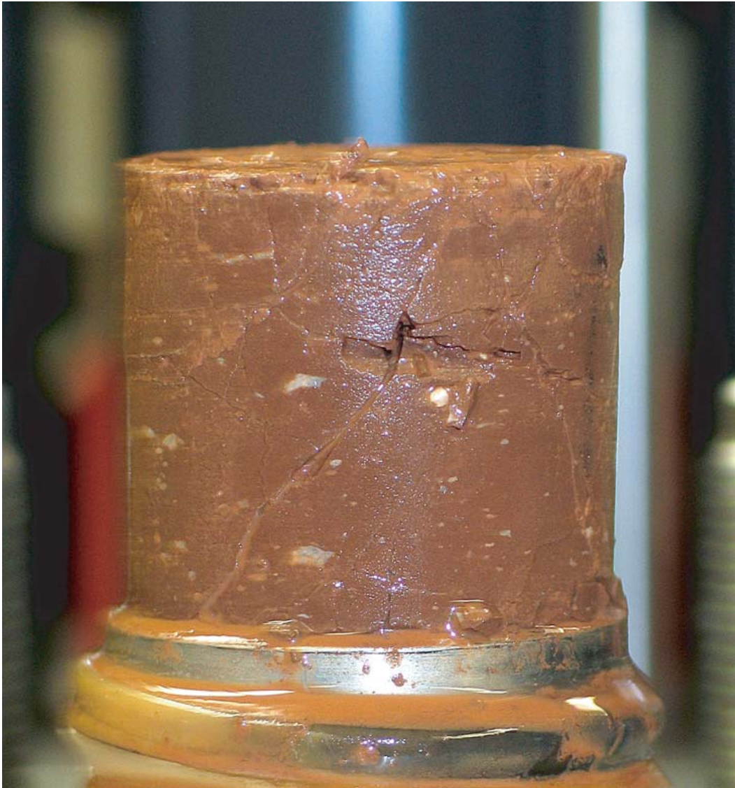
Figure 2.26: Cored claystone sample with irregular fractures after clastic behavior during a confined shortening test
