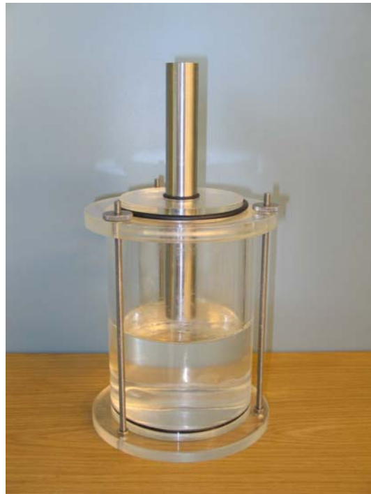
Figure 5.5: Testing device for small-scale convergence tests [6]
