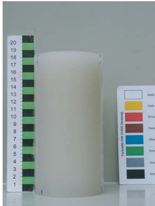
Figure 2.2: Cylindrical paraffin sample with ruler (cm) and reference color bar
