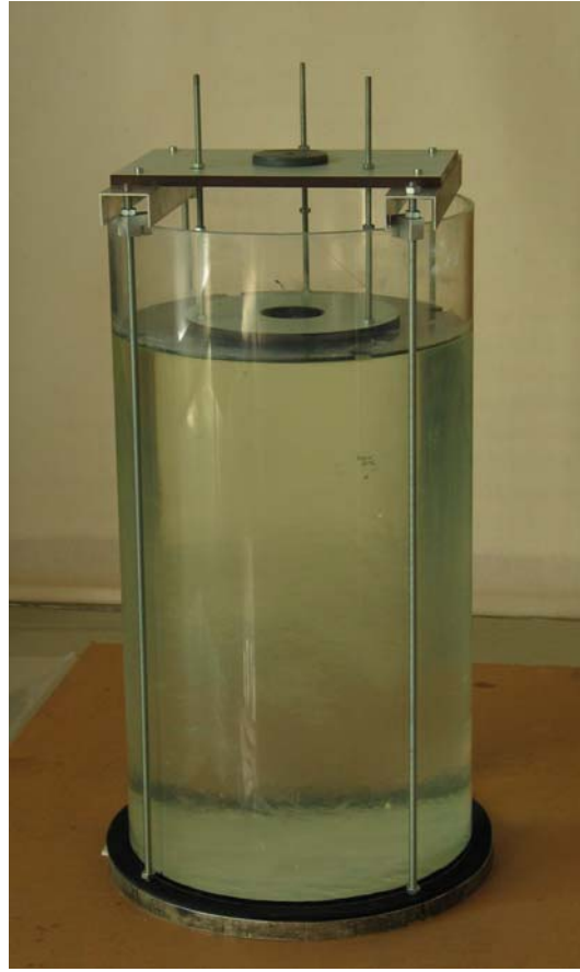
Figure 5.11: Testing device filled up with hydrogel [6]
