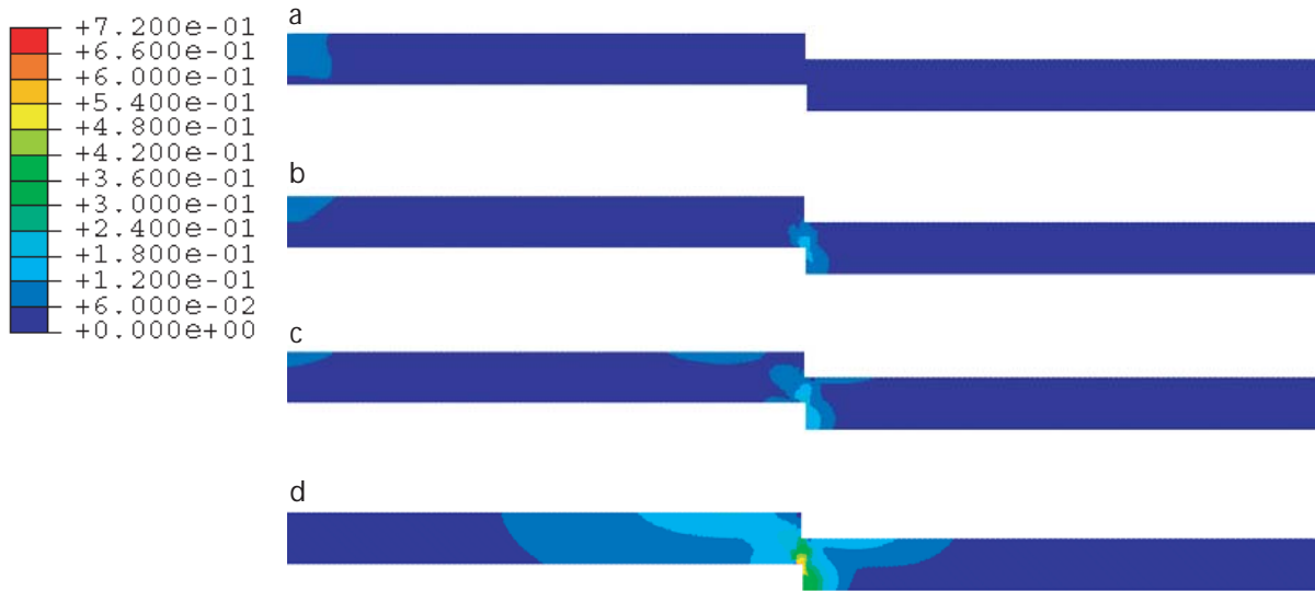
Figure 6.7: Induced deviatoric stresses \|\underline{T}^*\|/\Delta p_{max} in layer L3 (seal), results of numerical calculations with set 2 at the end of the calculation steps S1 to S4.
