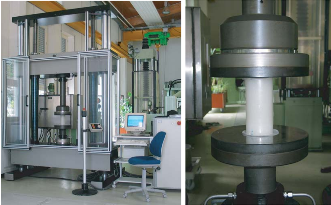
Figure 2.5: UTS testing device with cylindrical paraffin sample
