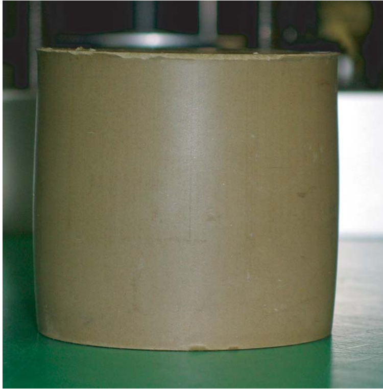
Figure 2.18: Deformed reconstituted bentonite sample after a confined shortening test up to an axial shortening of 16%
