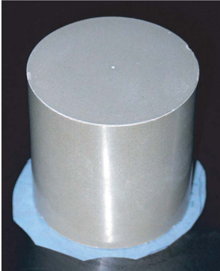
Figure 2.14: Reconstituted bentonite sample after compression with 150 MPa
