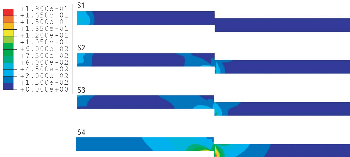
Figure 6.6: Induced deviatoric stresses \|\underline{T}^*\|/\Delta p_{max} in layer L3 (seal), results of numerical calculations with set 1 at the end of the calculation steps S1 to S4.
