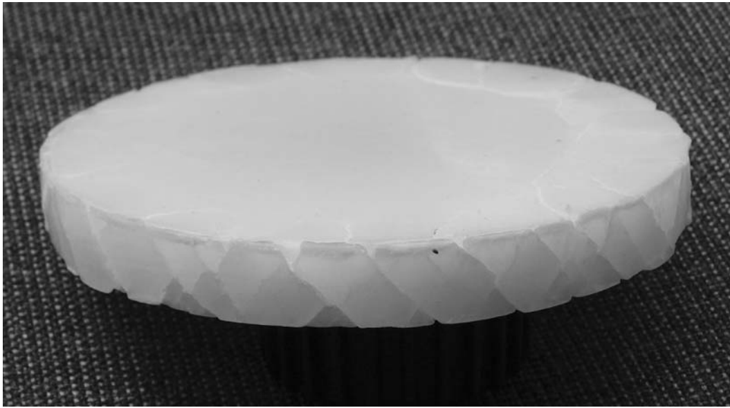
Figure 2.10: Shear band pattern of a flat paraffin sample after unconfined shortening with high axial shortening rate (courtesy K. Balthasar)
