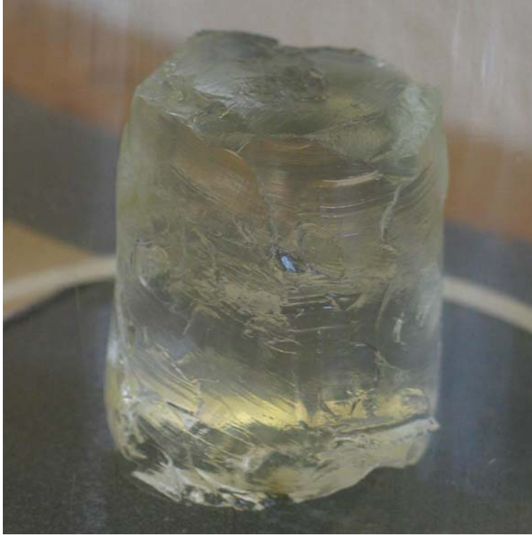
Figure 5.2: Cylindrical shape of the hydrogel sample at the beginning of the creep test ( h = 52 mm, d = 35 mm) [6]
