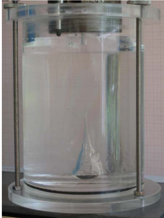
Figure 5.10: Enclosed air at the bottom after closure of the borehole at the end of a small-scale convergence test [6]
