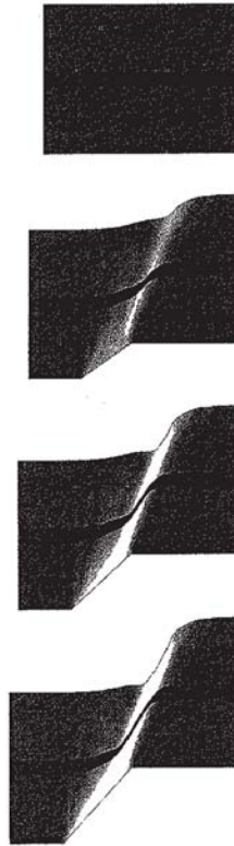
Figure 6.2: Simulated faulting with an arising clay smear, composite with dislocation, from [13]
