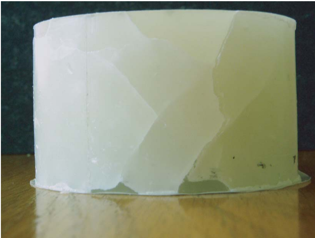
Figure 2.9: Evolution of helical shear bands with an unconfined shortening test with paraffin, courtesy K. Balthasar
