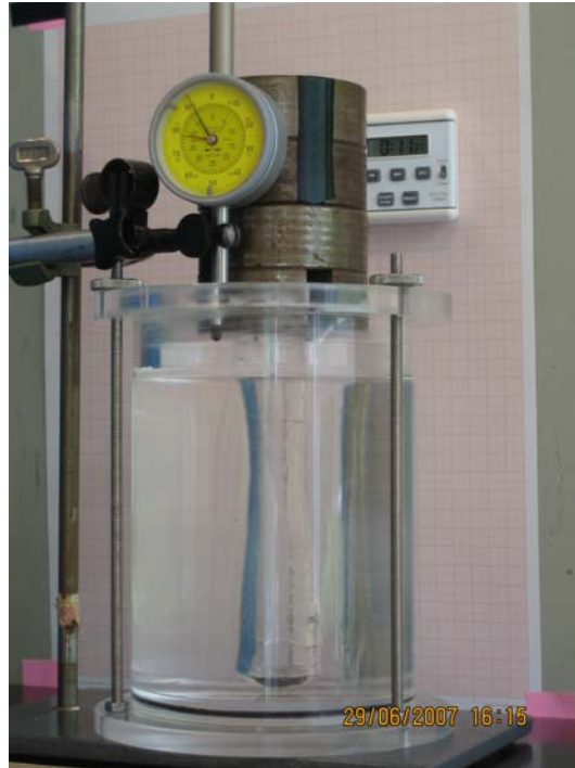
Figure 5.7: Operating testing device and convergence of the borehole during the small-scale test, [6]
