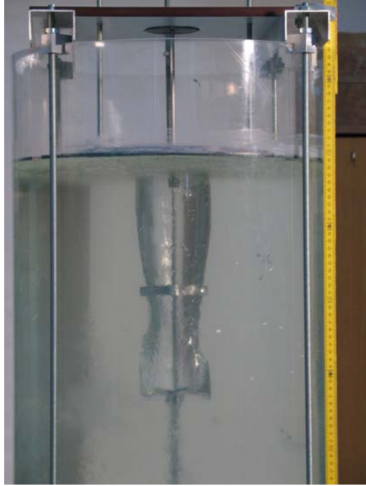
Figure 5.13: Deformation of the borehole immediately after removing the punching tube [6]
