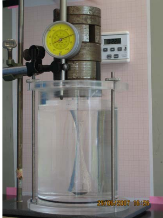
Figure 5.9: First closure in the middle third section of the borehole in a small-scale test [6]
