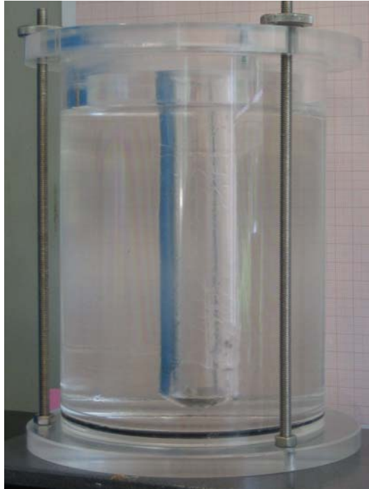
Figure 5.6: Circular vertical borehole at the beginning of a small-scale convergence test [6]
