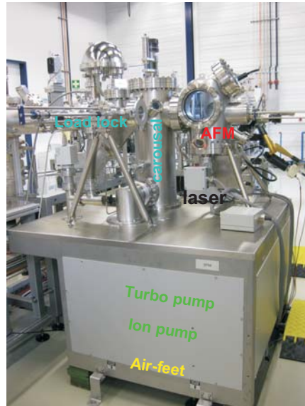
Figure 5.4 Large sample ultra-high vacuum AFM connected to the UHV analysis cluster at ANKA.
