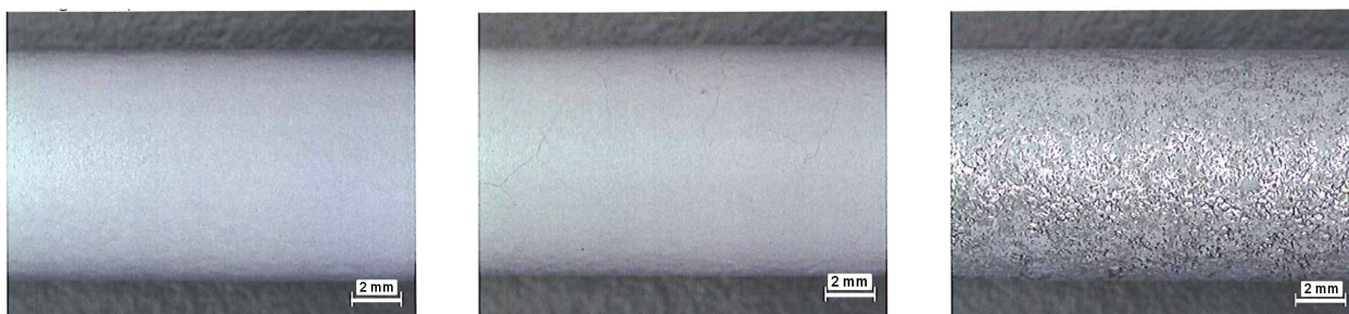
Figure 5.5.: Left: homogeneous porous layer; Middle: Cracks on layer show insufficient adhesion; Right: Melted layer caused by slightly higher local temperature
