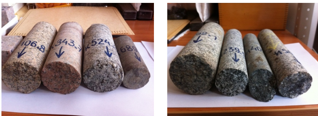
Figure 4: Rock samples to be granulated for sorption experiments from Kamenny (left) and Itatsky (right) areas.
