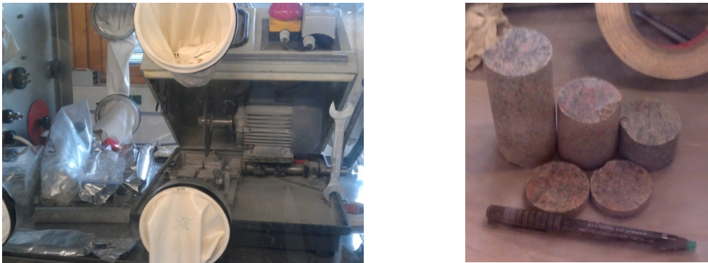
Figure 2: (left) Ar- glovebox equipped with the circular diamond saw for preparation of cores and discs of defined length. The crushed material and sieving procedure was prepared in the same box. (right) Äspö diorite cores of 10cm, 5cm, 3cm length and two discs of 1 cm thickness.
