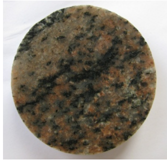
Figure 1: Sample AD1 for electromigration measurement.
