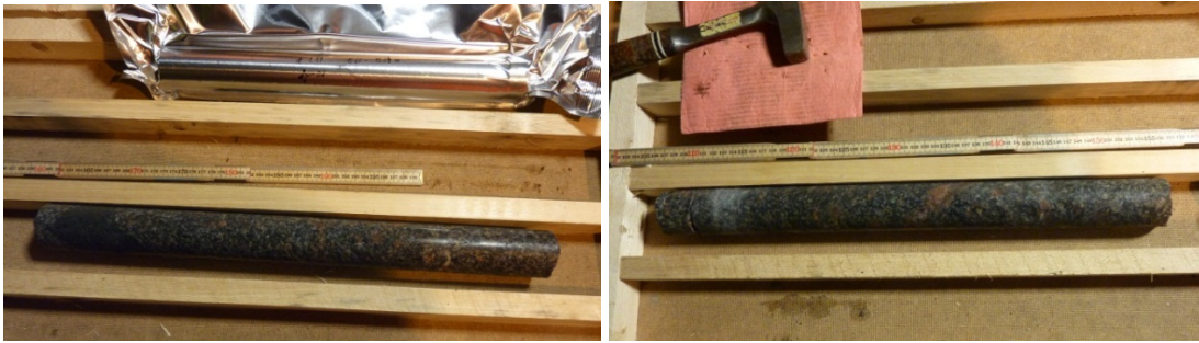
Figure 1: Photos of the Äspö diorite (ÄD) cores #1.32 (left) and #1.33 (right) directly taken after drilling subsequently used for preparation of crushed material.
