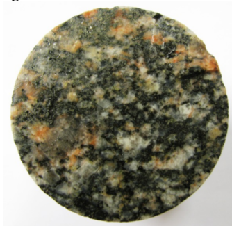
Figure 1: Sample AD1 for electromigration measurement.
