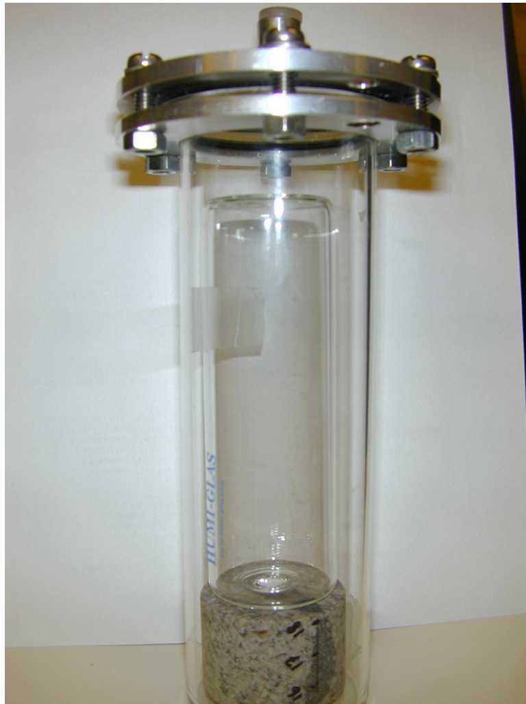
Figure 1: The specially made holder for gas adsorption measurements of 3cm drill-core sections.
