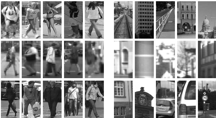
Figure 27.2: Five positive (left) and negative (right) samples from each dataset: INRIA (top), DaimlerChrysler (middle) and TUD-Brussels (bottom).
