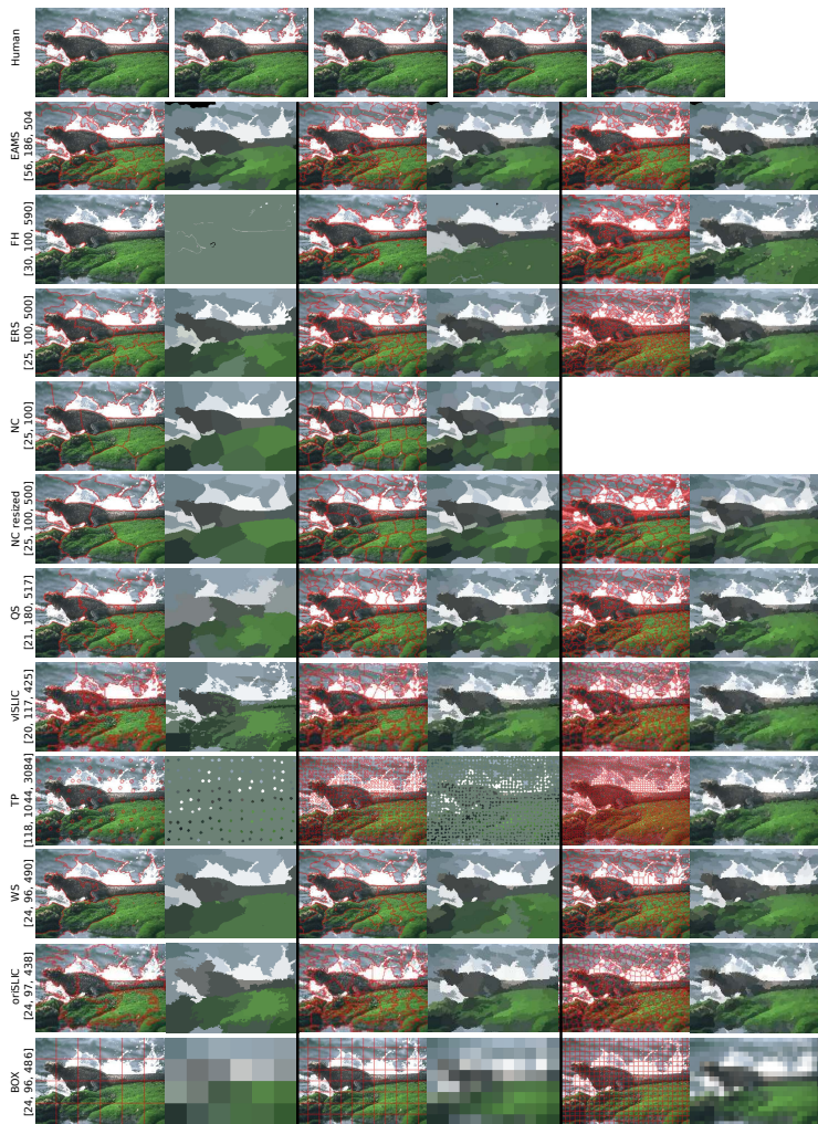
Figure 18.7: Superpixel segmentations. ( top-row ) Different segmentations by humans taken as ground truth. ( other rows ) Each row shows results of one algorithm and 3 parameter settings, visualized as overlaid boundary image and superpixels with average image colors. The algorithms parameters were chosen to produce about 25, 100 and 500 superpixels (except for TP and NC). The algorithm name and individual number of superpixels are given on the very left.
