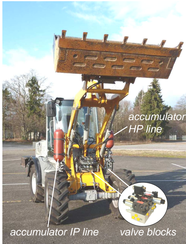
Figure 10: Results Test machine with mounted valve blocks and accumulators
