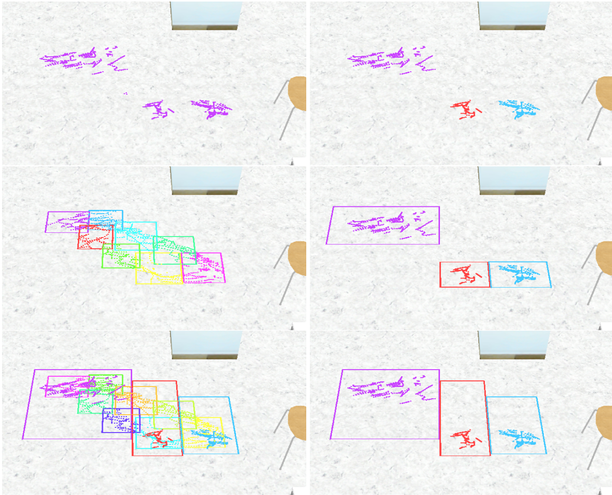
Figure 4.6.: From top left to bottom right: standing data for clustering, data clustered with DBscan, k-means clustered transition regions, regions without transitions, regions including transitions and final regions. - [147]
