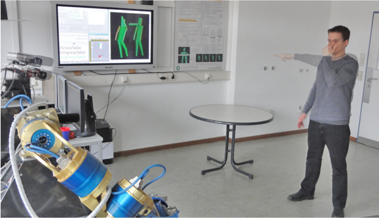
Figure 4.2.: Illustration of the attention mechanism consisting of two special gestures: first pointing at the own eyes and then left or right. - [125]
