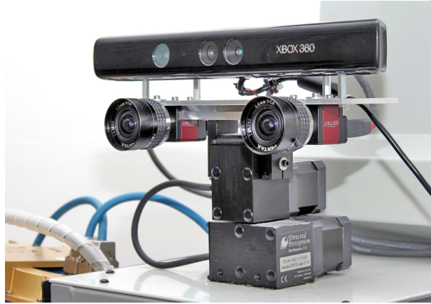
Figure 3.3.: Camera head of Albert with pan-tilt unit (neck), Kinect 3D depth camera and Guppy stereo color cameras. - [125]
