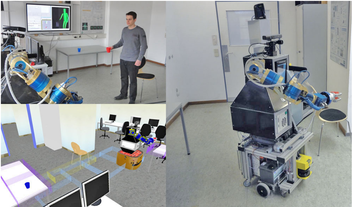
Figure 5.3.: Illustration of CESM-2 during transport of the cup after pulling the chair out of the way. Shown clockwise: execution, visualization of feature states and demonstration. - [125]
