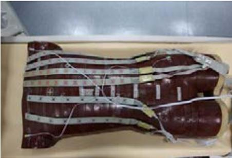
(b) active electrode strips on phantom
