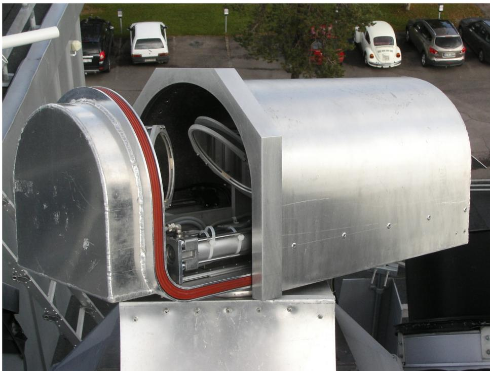
Figure 5.1: Tracker in Kiruna on the roof of the IRF building. The letter-box cover can be moved by pressurized air, which is also used to inflate the red sealing.
