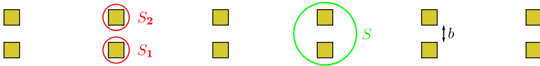
Figure 7.41: For small layer spacings b , describing the problem with one scattering matrix rather than with two appears reasonable. Then, we describe the system as one layer of double-rods instead of two layers of rods.
