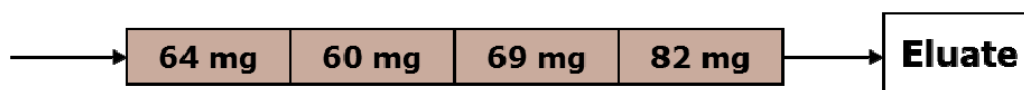
Figure 44: Scheme for the post mortem analysis of Eu(III) in the eluate and in four clay pieces from a recovered OPA-column bloc after a long time migration experiment
