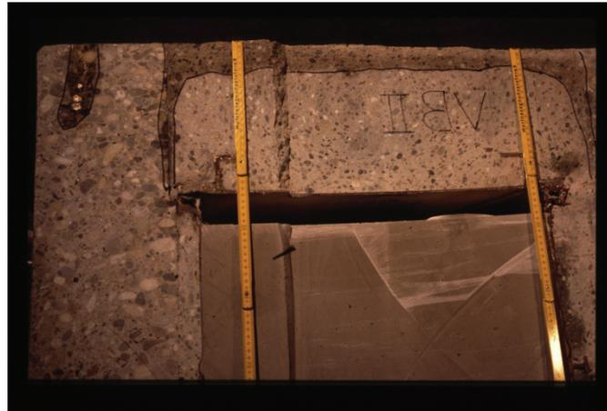
Fig. 14 Cut through a cylindrical self-shielded concrete disposal container after corrosion in saturated  $\text{MgCl}_2$  solution (Q brine) for 11 yrs.
