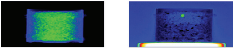
Figure 23.4: The resulting BMD images, calculated from the images in Fig. 23.3, are shown in color. The left image represents the kimberlite content. The right image represents the carbon content and the diamond can be seen clearly.
