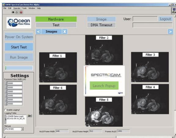
Figure 9.3: SpectroCam by PIXELTEQ live view screenshot. The six channels refresh constantly to provide a live view of the samples. Filters with approximately 100nm bandwidths spanning from 1050nm to 1700nm were utilized.
