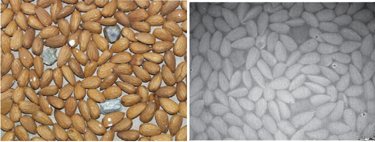
Figure 12.3: Photographic (left) and infrared (right) image of almonds with stones as foreign bodies.
