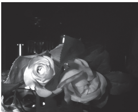
Figure 9.4: Image from filter 5 in PIXELTEQ SpectroCam MSI camera, corresponding to 1500nm-1600nm. Note the real rose on the left shows stronger signal (indicated by greater pixel intensities) in the 1500-1600nm range.
