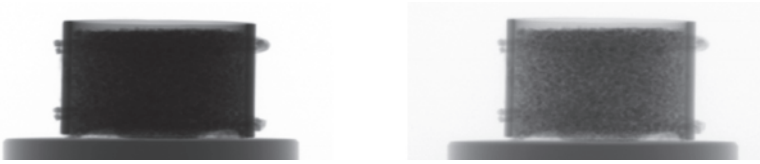
Figure 23.3: The two images show the example of the diamond embedded in granulated kimberlite at two different spectra (80 kV and 120 kV).
