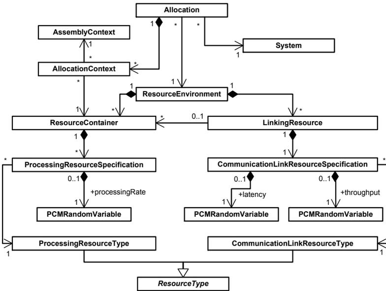
Figure 2.22: Meta Model of PCM Allocation Model and Resource Environment
