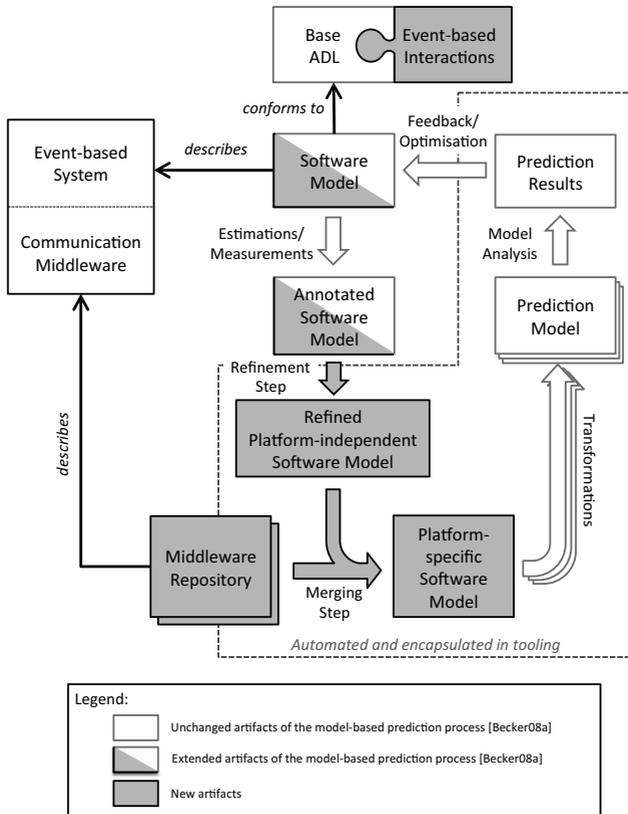
Figure 1.1: Extended Model-based Performance Prediction Process
