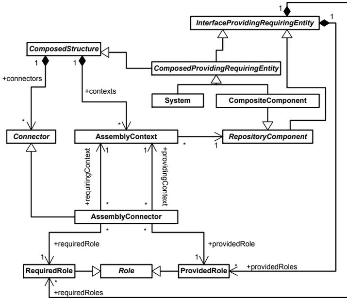
Figure 2.21: Meta Model of PCM System Model
