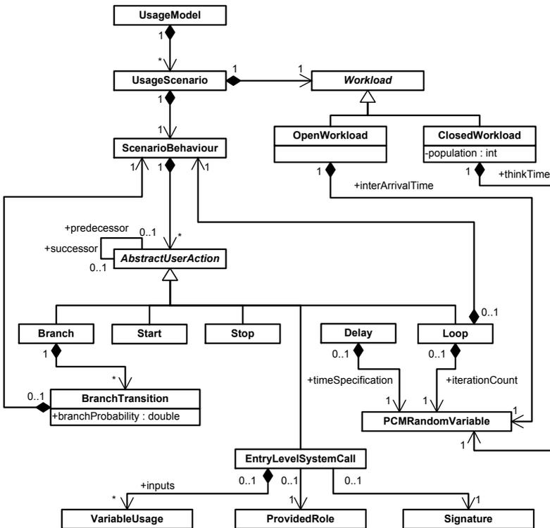
Figure 2.23: Meta Model of PCM Usage Model
