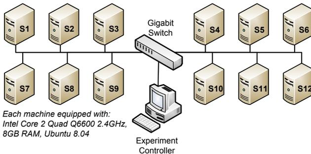
Figure 6.4: Experimental Environment of the Traffic Monitoring System
