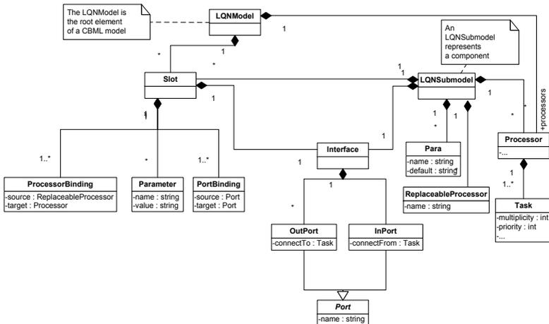
Figure 2.17.: Excerpt of the CBML Metamodel, Extracted from the XML Schema
