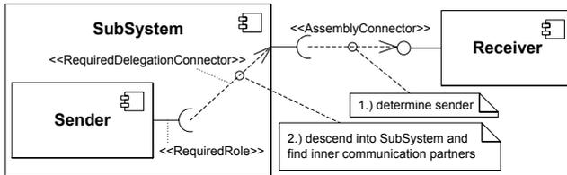
(c) Case 3: The Communication Partner is Contained in a SubSystem which is not Allocated as a Whole
