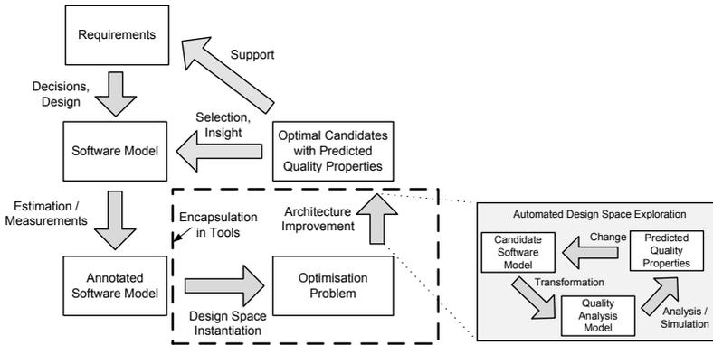
Figure 1.2.: Model-based Architecture Improvement Process with Feedback into Requirements Engineering
