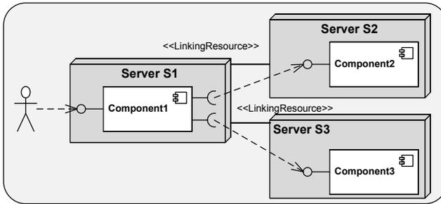
Figure 6.5.: Simple Example with Partially Connected Servers
