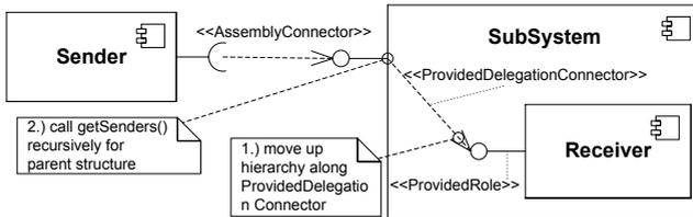
(b) Case 2: Current Component is Contained in SubSystem and Connected to SubSystem Roles
