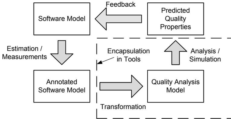
Figure 1.1.: Traditional Model-based Quality Prediction Process (adapted from (H. Koziolok, 2008))
