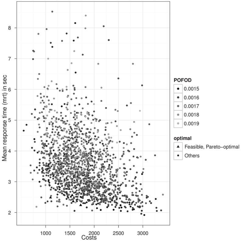
Figure 9.24.: Result of an Optimization Run  $MC_0$  with medium requirements  $scen = M$  and the Constrained Tournament Method  $c = C$ .
