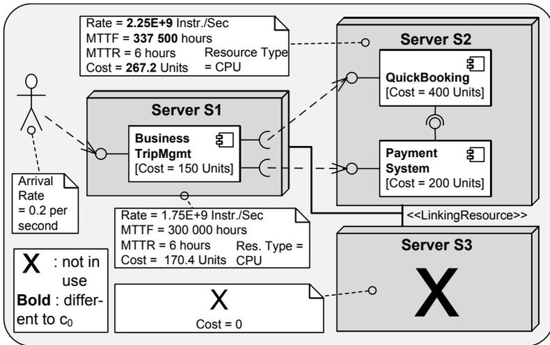
Figure 8.4.: Example PCM Model for Pareto-optimal Candidate  $c_6$  would improve the current results, and stop the search if this is not expected. Such criteria are discussed in Section 8.2.6.
