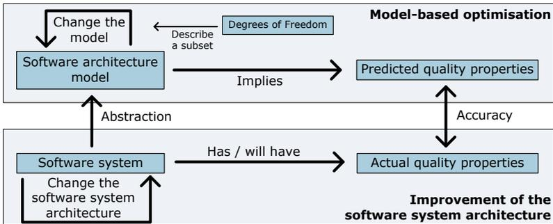
Figure 5.5.: Model-based Software Architecture Optimization
