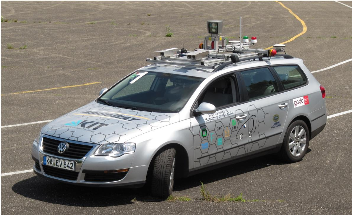
**Figure 1.1:** The experimental car *AnnieWAY* is equipped with numerous sensors and is capable of driving autonomously. The presented work focuses on data from the top mounted laser scanner and targets at sensing the environment.
