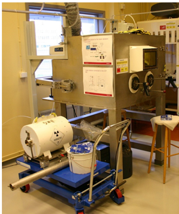
Figure 3: The laser ablation hot cell and the sample transfer cask
