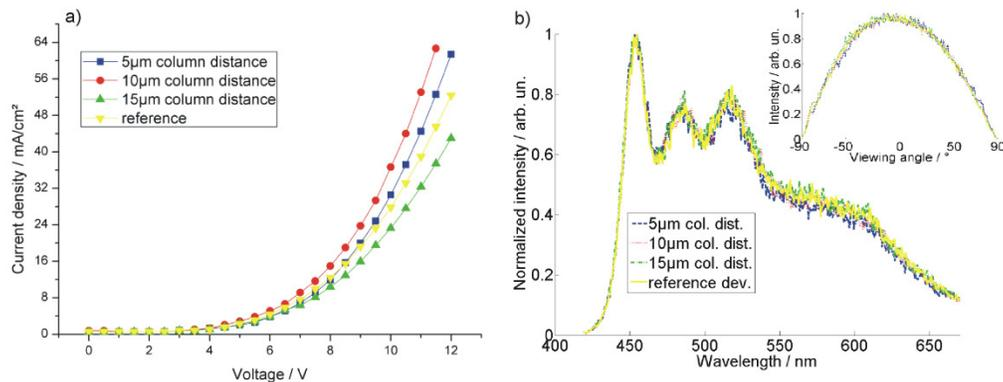
Fig. 3. (a) Current-density characteristics of devices with different column distances and a column height of 66 nm. (b) Emission spectra at a viewing angle of  $40^\circ$ . The inset shows the angle resolved emission at a wavelength of 520 nm.
