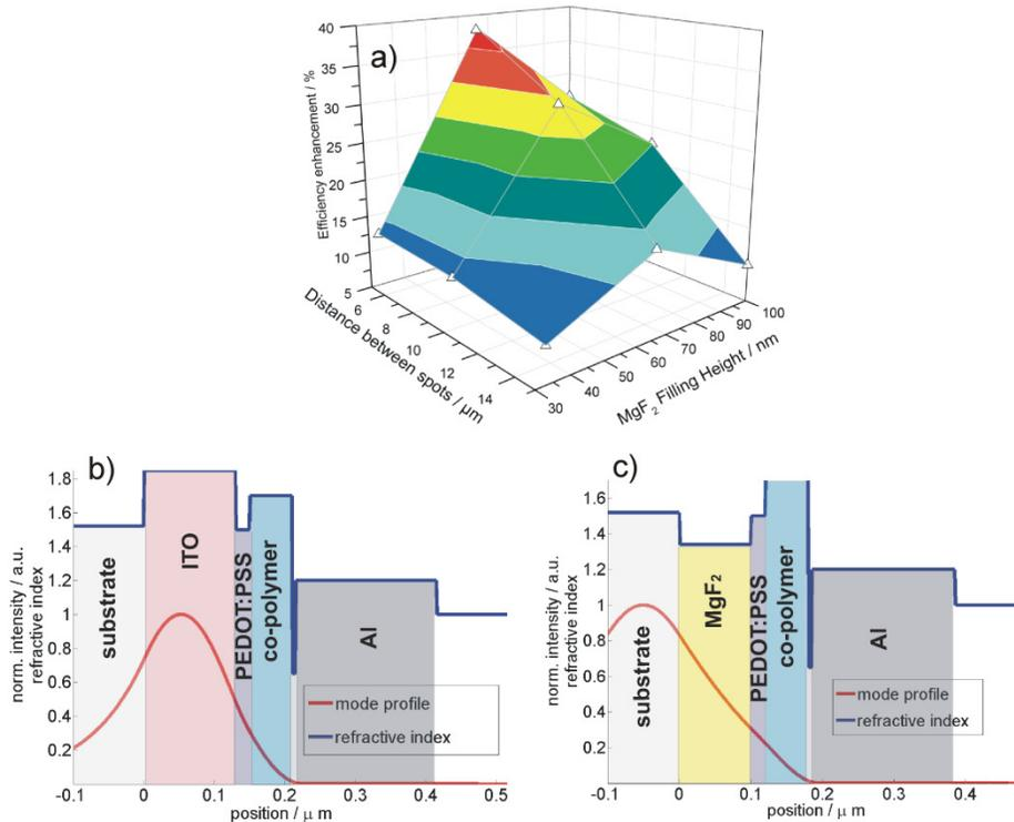
Fig. 2. (a) Measured efficiency enhancement with different column distances and heights. (b) T-Matrix simulation of the waveguide mode at  $450\ \text{nm}$  distribution at the position of ITO. (c) T-Matrix simulation of the waveguide at  $450\ \text{nm}$  mode distribution at the position of  $\text{MgF}_2$ . The waveguide mode is shifted towards the substrate.
