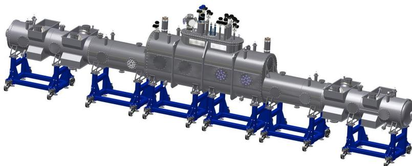
**Figure 2.6:** The windowless gaseous tritium source consists of a 16 m long cryostat containing the beam tube. This 90 mm beam tube is kept on a stable temperature by a 2-phase neon cooling system
