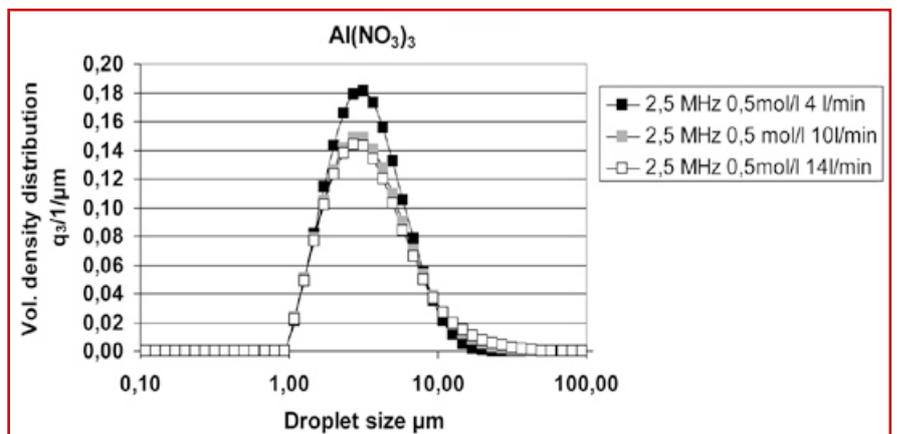
Fig. 7: Influence of carrier gas ( $N_2$ ) flow rate on droplet size distribution in case of  $Al(NO_3)_3$  ultrasonic spray formation
