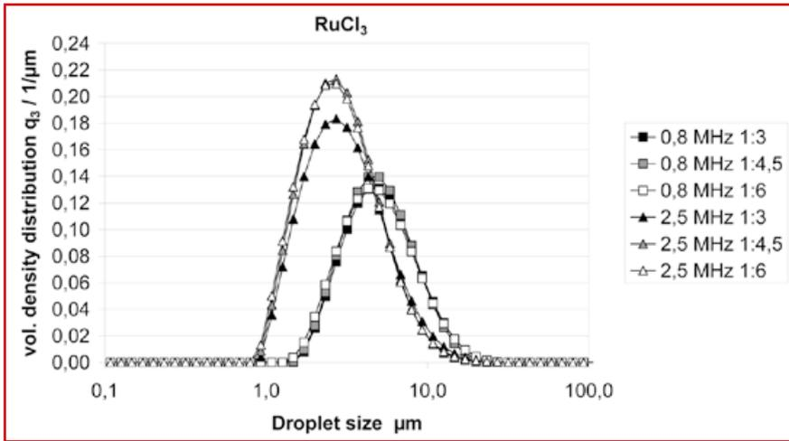
Fig. 5: Dependence of droplet size distribution from ratio of precursors in solution ( $RuCl_3:C_{16}H_{36}O_4Ti$ ) and ultrasonic frequency
