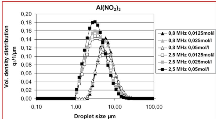
**Fig. 3: Dependence of droplet size distribution from concentration of  $\text{Al}(\text{NO}_3)_3$  precursor solution and ultrasonic frequency**
