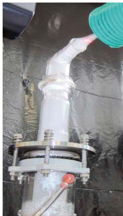
**Fig. 1: Aerosol production by an ultrasonic generator**
