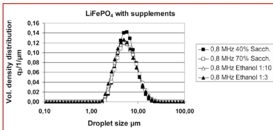
**Fig. 8: Influence of surface active ethanol as well as sugar addition to the 0.05 mol/l Li-precursor solution on droplet size distribution**
