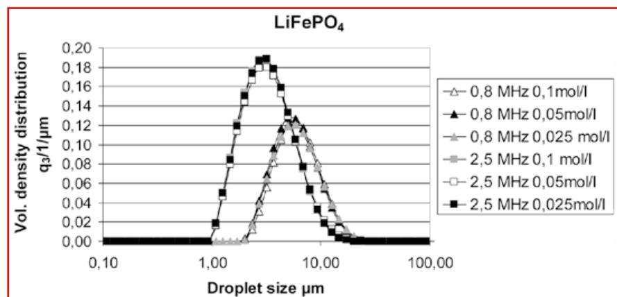
**Fig. 4: Dependence of droplet size distribution from concentration of  $\text{LiFePO}_4$  precursor solution and ultrasonic frequency**
