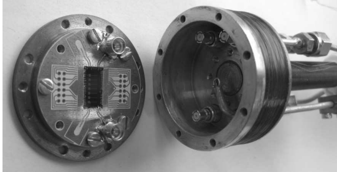
Figure 3.3: Photograph of the cryogenic sample compartment. The external coil wound around the box is used to supply a homogeneous flux bias to the qubits. A ring of holes close to the center holds the gradient coils (see section 3.2.2) which are not installed here. The SMP-type microwave connectors are threepartite to provide a low mismatch even when the PCB is not perfectly aligned. The small loop terminating the microwave cable in the center of the picture, used to supply nanosecond flux pulses to the qubits, was only present in one of the runs.
