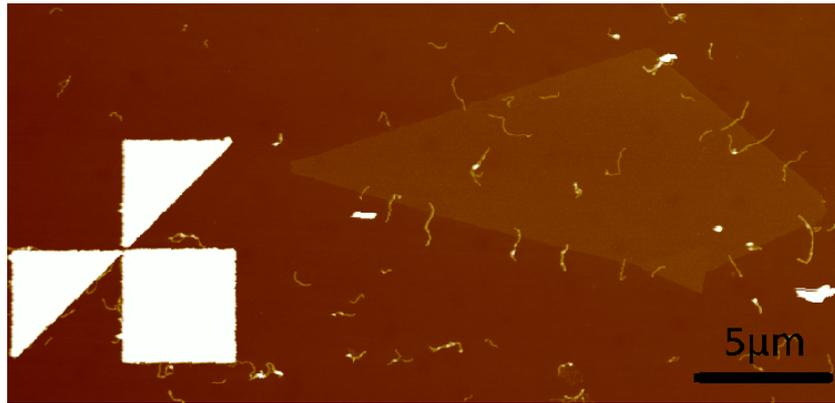
**Figure 6.13:** AFM picture of a sample ready for the lithography step. 11 MWCNT have been dragged off onto the graphene flake. On the left side, an alignment marker is visible.
