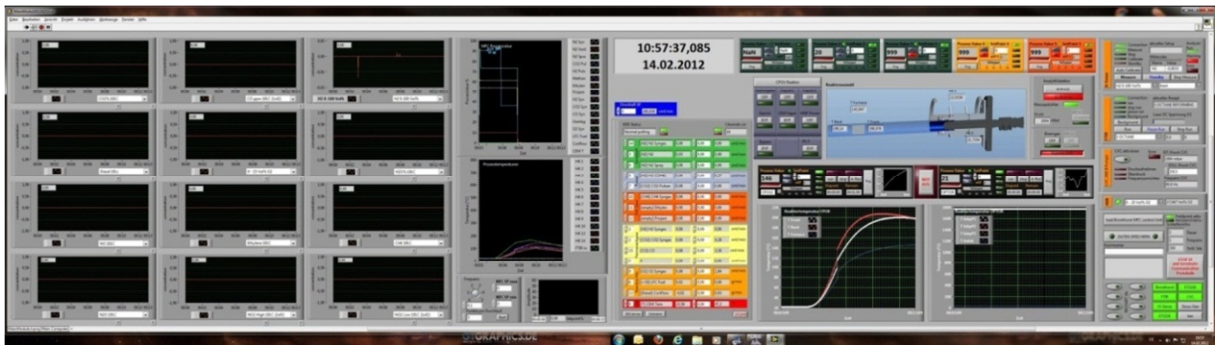
Figure 4-5: Screenshot of the LabView® GUI. Left-hand side shows the online process value signal curve diagrams. Right-hand side shows the control panels for MFCs, TICs, valves, and signal curves for temperature control, data storage, and analytic devices.
