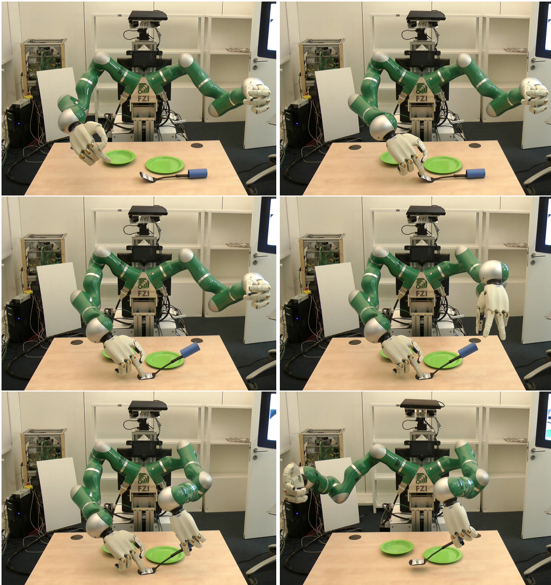
Figure 5.48.: Lifting a spoon: execution on Adero. The handle of the spatula was enlarged to be able to detect the spoon visually and grasp it securely. - [53]
