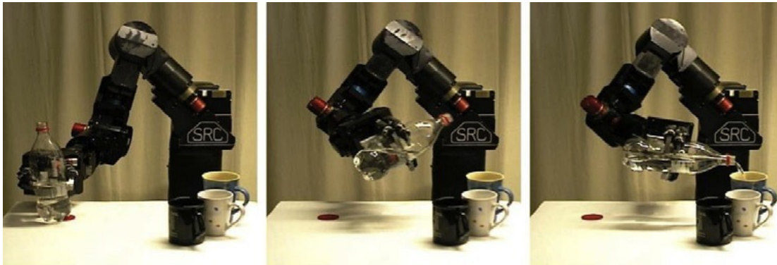
(c) Reproduction using a 6-DOF Sarcos master arm with identical kinematics.
