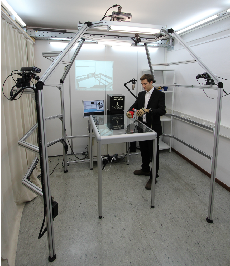
Figure 1.3.: Sensor environment with magnetic field trackers, datagloves, tactile sensors and two robot heads featuring a stereo camera, a RGB-D camera and a pan-tilt-unit.
